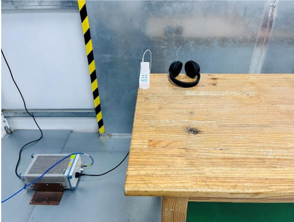
AC Power Line Conducted Emission
