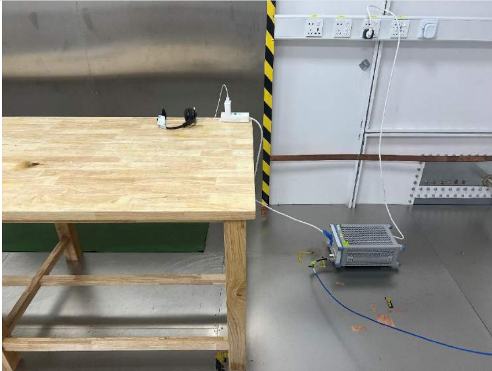
AC Power Line Conducted Emission
