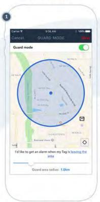
Zoom and slide the map to select the Guard Zone radius. "Leaving" or "Entering the area" criteria can be switched by clicking on the link at the bottom. Guard zone alerts are coming as notifications on your smartphone and are triggered only by the GPS coordinates.
