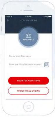
Click "+" on the top left of the main screen to register the new iTraq device. Give it a name, add photo and enter the serial number or click QR code button to read it off the device sticker with your phone camera.
