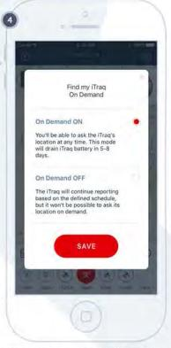
When you turn OnDemand mode ON, in addition to scheduled reports, you can ask for the device location at any time. Please note that turning this mode on will significantly reduce the battery life of the device.
