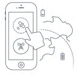
In the iTraq mobile application you can choose which location technology will be used by iTraq: GPS (accurate, outdoors, shorter battery life) or Cell-ID (not accurate, indoors, longer battery life). If iTraq cannot get the GPS data it will revert to Cell-ID data.
