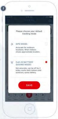
Switch between default location tracking technology. Device will report CEII-ID or GPS location at the schedule that you set. When GPS is selected, but the device doesn't see the satellites, CeII-ID coordinate will be sent as a fall back tech.
