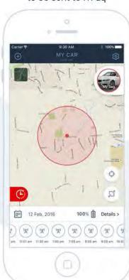
Once you made changes to the device settings (Schedule, OnDemand, Guard zone, GPS vs Cell-ID etc..), you will see this red spinning watch icon on the screen. It will be present until the new info is sent to the device.
