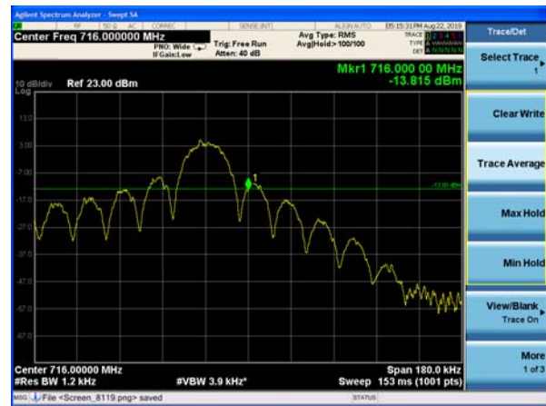
NB-IOT Band 12 QPSK 15kHz 12@0 CH-High
