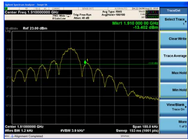
NB-IOT Band 2 QPSK 15kHz 12@0 CH-High
