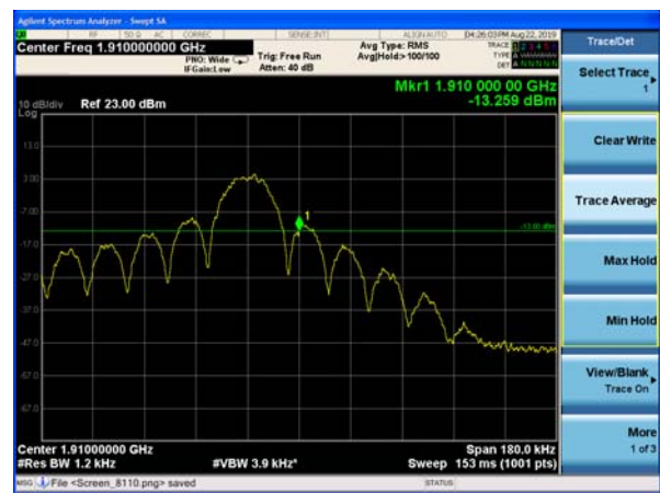
NB-IOT Band 2 QPSK 3.75kHz 1@47 CH-High
