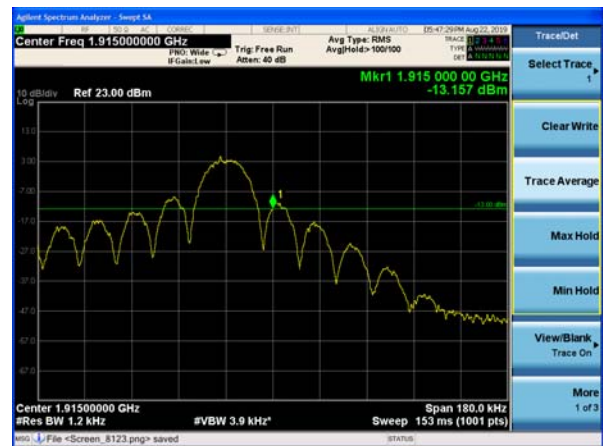
NB-IOT Band 25 QPSK 15kHz 12@0 CH-High
