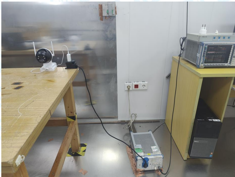
Photo of Setup for Conducted Emission-X30
