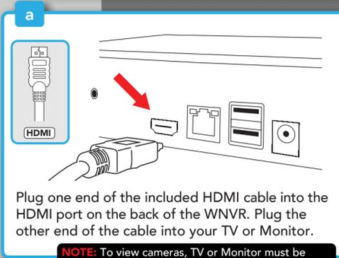
Plug one end of the included HDMI cable into the HDMI port on the back of the WNVR. Plug the other end of the cable into your TV or Monitor.
