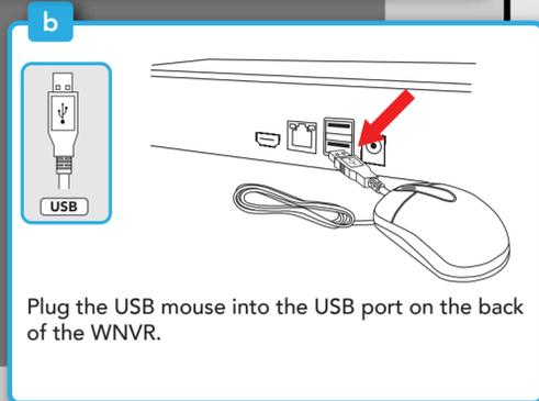
Plug the USB mouse into the USB port on the back of the WNVR.
