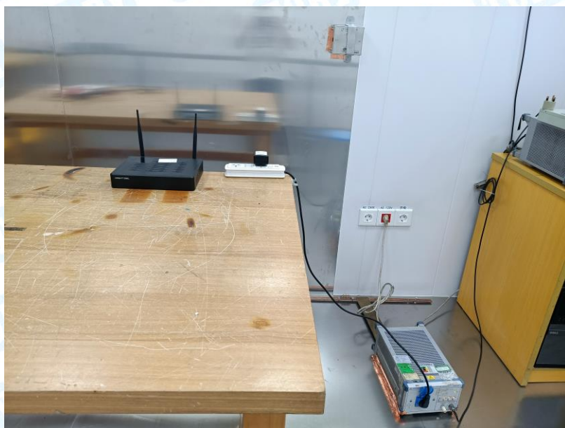
Photo of Setup for Conducted Emission
