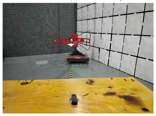
Radiated Emissions, Above 1GHz Test Setup
