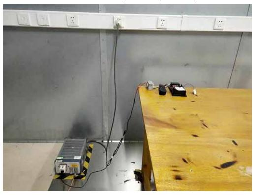
Radiated Emissions, 9kHz to 30MHz Test Setup
