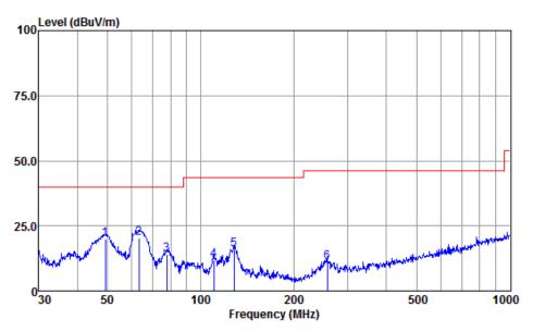
Antenna Polarity :VERTICAL EUT/Project :2997CR Test mode :b
