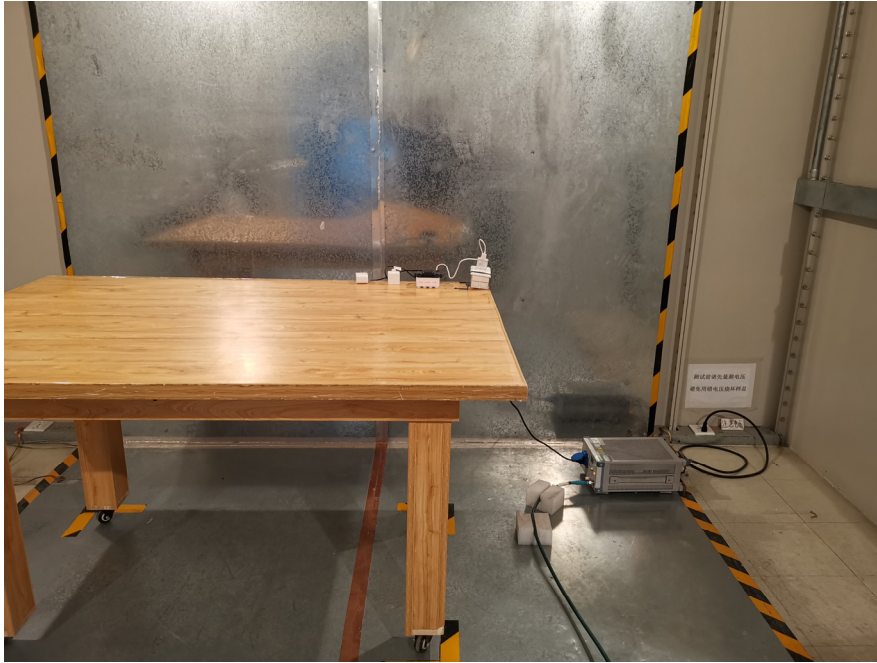
Conducted Emissions - Rear Side
