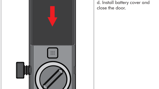
d. Install battery cover and close the door.
