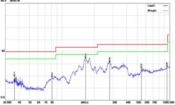
Note: The charging of < 1% Battery, 50% Battery, >99% Battery all has been tested, the worst case is charging of < 1% Battery, only shown the worst case in this report.
