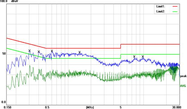
Note: The charging of < 1% Battery, 50% Battery, > 99% Battery all has been tested, the worst case is charging of < 1% Battery, only shown the worst case in this report.
