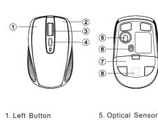
6. Power Switch 7. Battery Cover 8. USB Receiver (Built-In)
