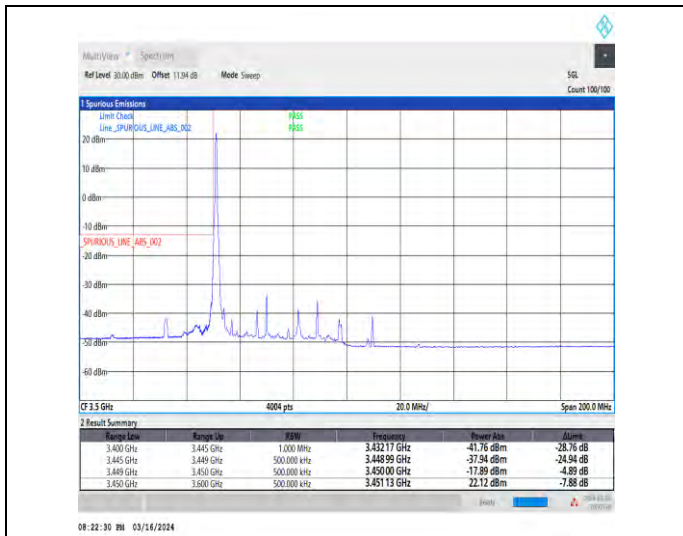
1-N77-3450-3550-30-40-L-1-DFT-PI2BPSK-Edge_1RB _Left-1@0-Ant3-1--PASS-see graph
