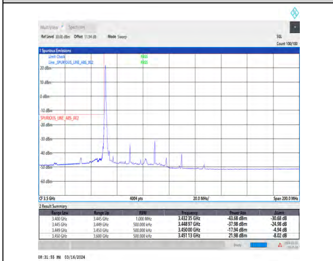
1-N77-3450-3550-30-40-L-4-CP-QPSK-Edge_1RB_Lef t-1@0-Ant3-1--PASS-see graph
