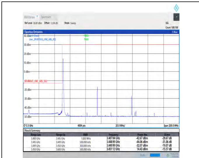
1-N77-3450-3550-30-90-L-1-DFT-PI2BPSK-Edge_1RB _Left-1@0-Ant3-1--PASS-see graph
