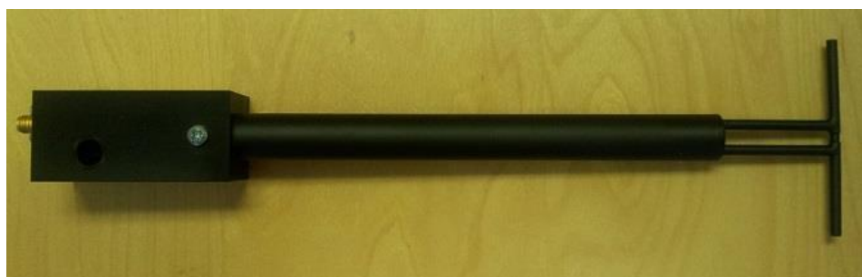
Figure 1 – MVG COMOSAR Validation Dipole
