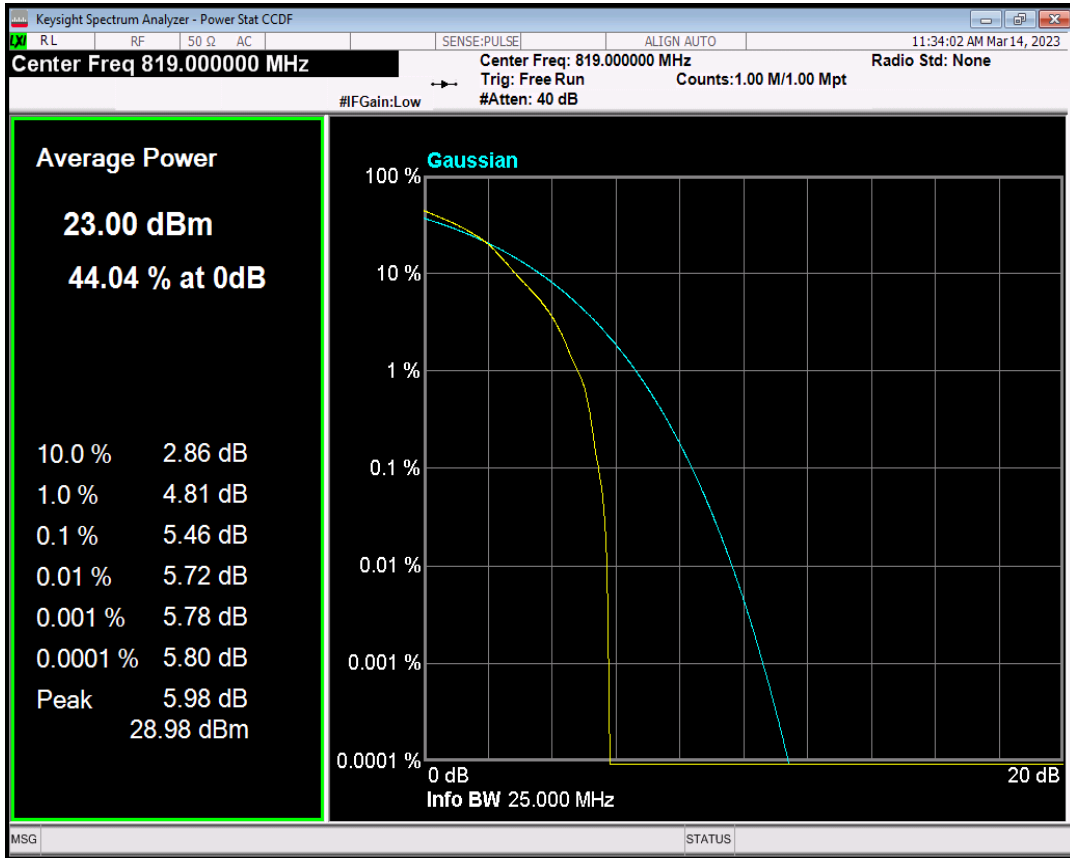
Band26(824-849) QPSK BW=1.4MHz Channel=26915 RB Size=1 Position=#0
