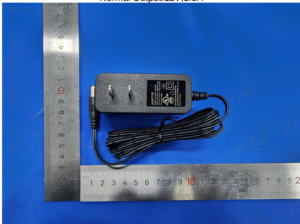
Model Name: AT-397A-120150A Input: 100-240V~,50/60Hz,0.5A Normal Output:12V,1.5A
