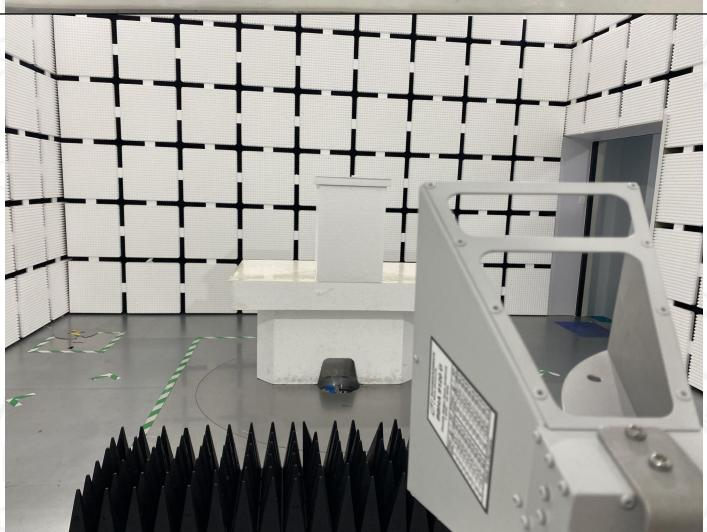
A photograph of an antenna mounted on a turntable inside a large anechoic chamber. The chamber walls are covered with a grid of metal mesh panels. The floor is a light-colored concrete. In the foreground, a black, spiky absorber panel is visible. The BTEK logo and Chinese text '邦泰检测' are visible on the wall. |
