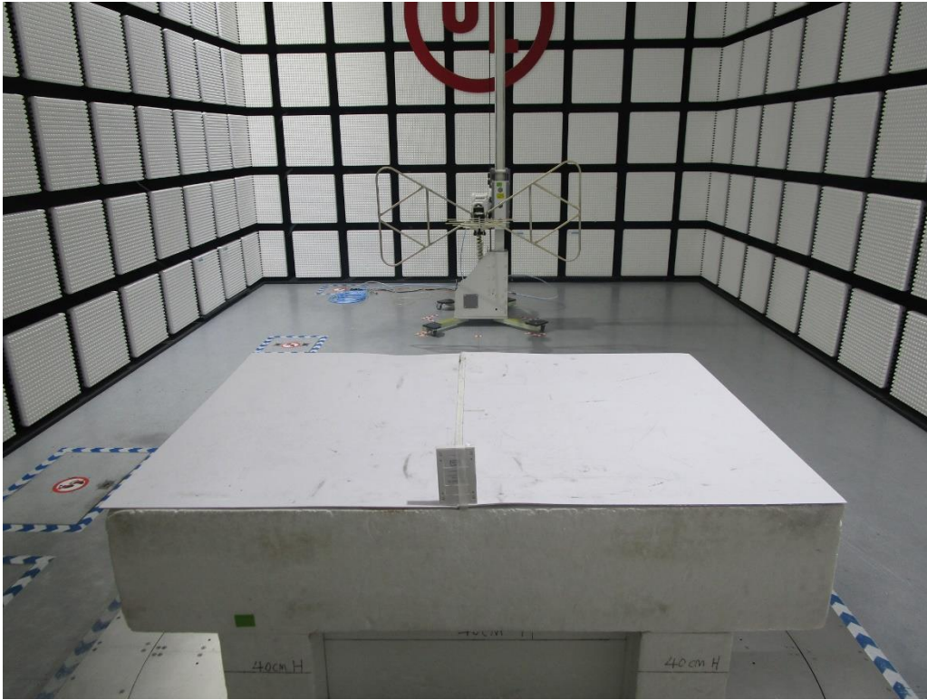
Radiated Disturbance Setup Below 30 MHz
