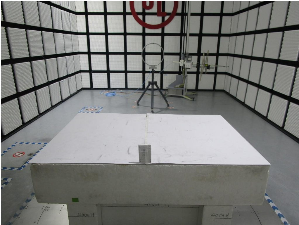
Radiated Disturbance Setup Below 30 MHz
