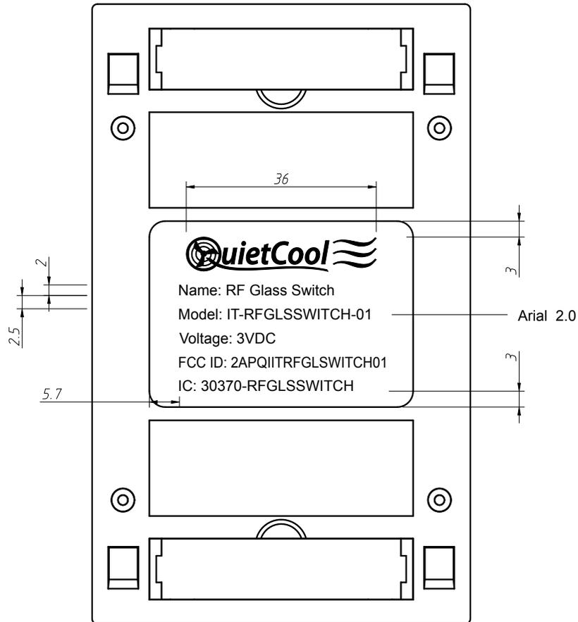
note:the label is on the back of the device through silk-screen printing.
