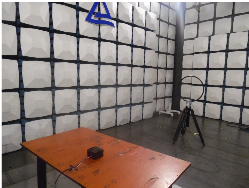
Photograph 1: Set-up for Radiated Spurious Emission, 9kHz - 30MHz
