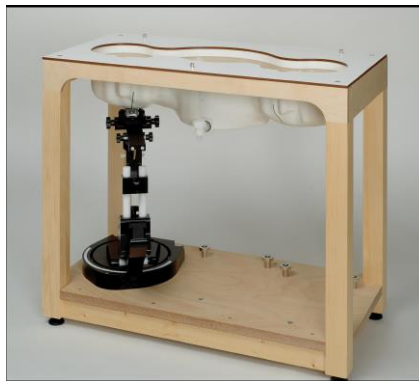
Picture C.10: SAM Twin Phantom
