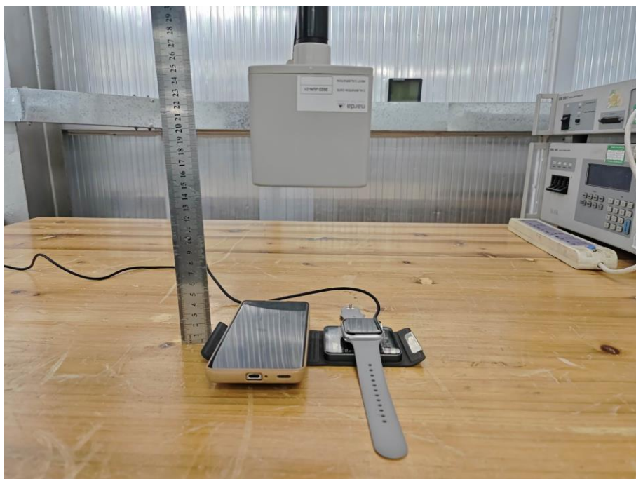
Test Position F-20cm from the edge of EUT to the geometric center of the probe
