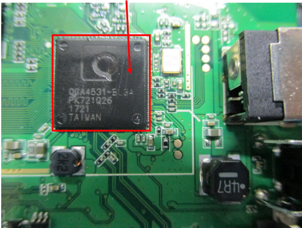
WIFI Chip IC – Top View
