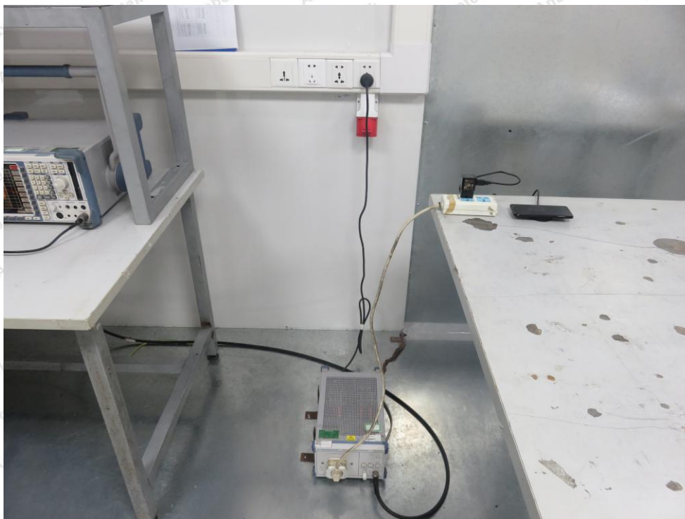
Photo of Conducted Emission Measurement
