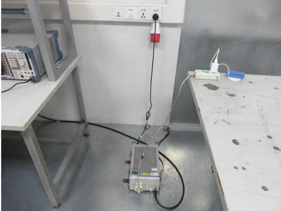
Photo of Power Line Conducted Emission Test
