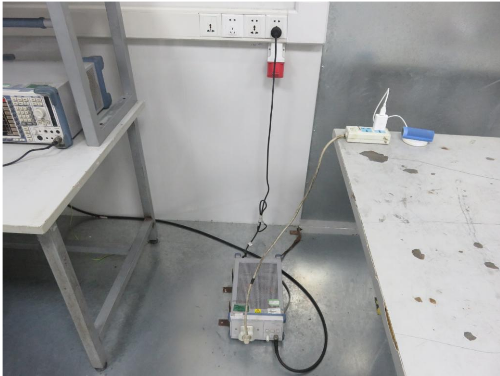
Photo of Power Line Conducted Emission Test
