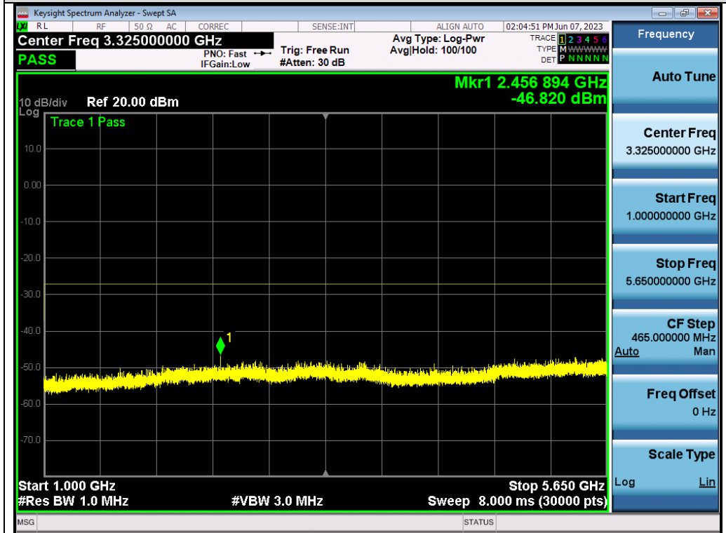
Test_Graph_802.11a_ANT1_5745_6Mbps_Frequency Band2
