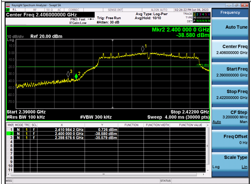
Test_Graph_802.11g_ANT1_2412_6Mbps_Lower Band Edge Emissions
