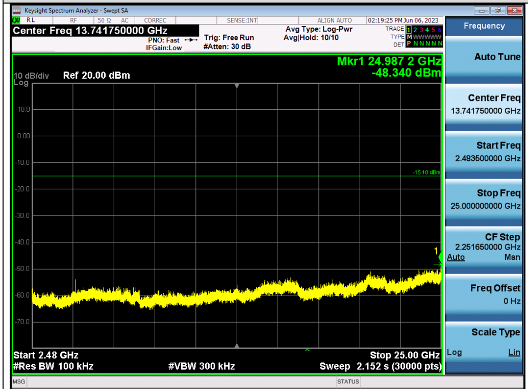
Test_Graph_802.11b_ANT1_2437_1Mbps_Higher Band Emissions
