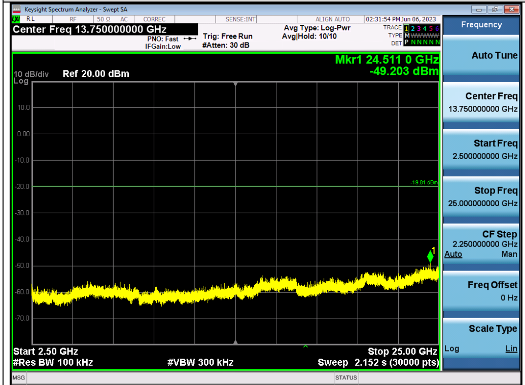
Test_Graph_802.11g_ANT1_2462_6Mbps_Higher Band Emissions
