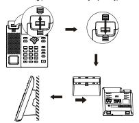
Note: The installation height of the wall-mounted bracket is less than 2 meters from the ground.
