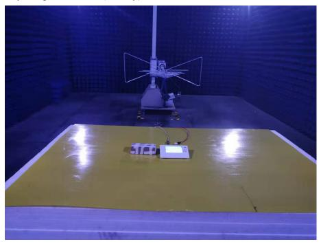
Photo of Radiated Emission Measurement (Above 1G)
