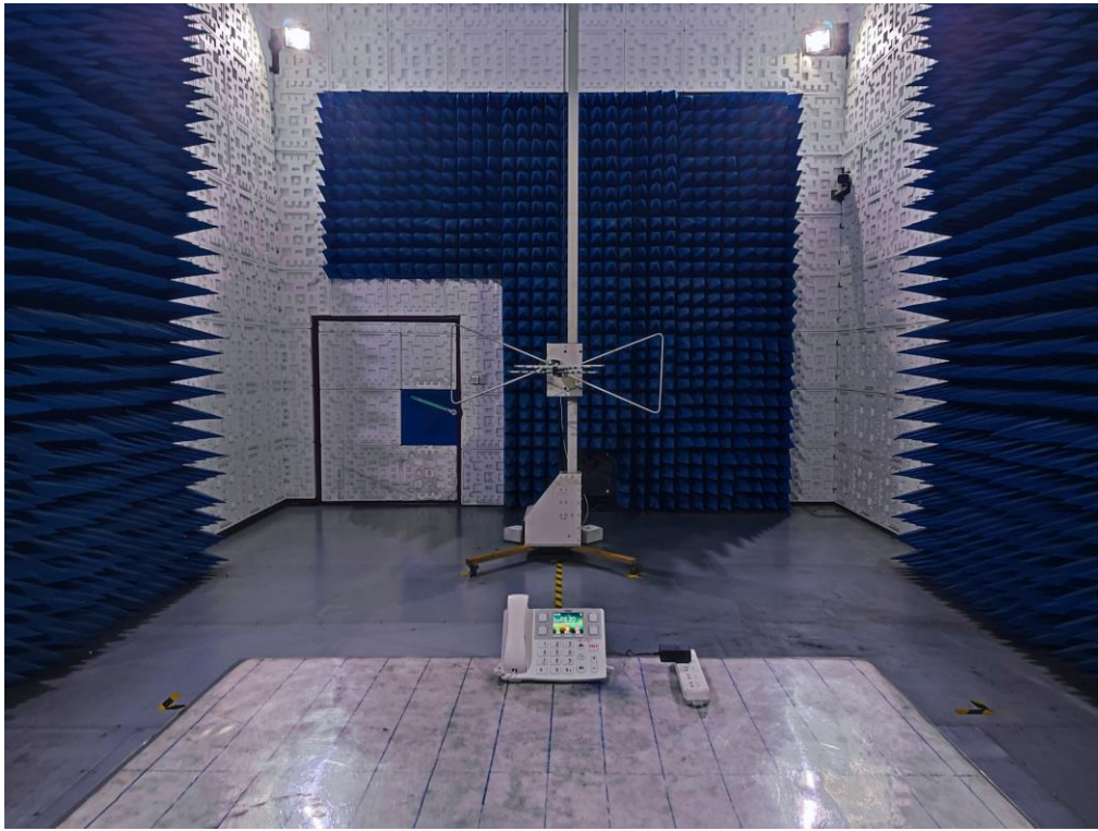
RADIATED EMISSION TEST SETUP ABOVE 1GHz (by Adapter)
