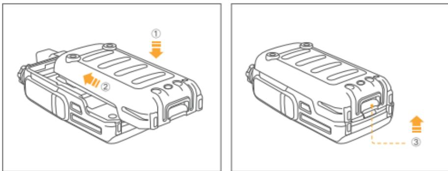
To install the battery, put the battery on the back of the radio, as shown in ①②. Push it horizontally along the slot to the top until it clicks.
