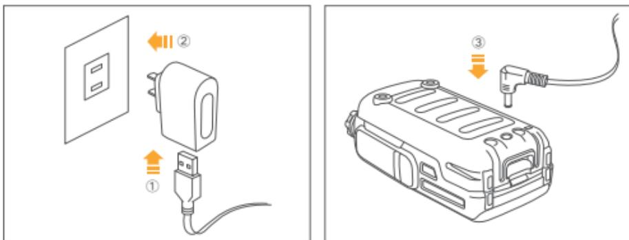
1. As ①② shown, connect the charging cable to the power adapter, then connect the power adapter to the AC power outlet.
