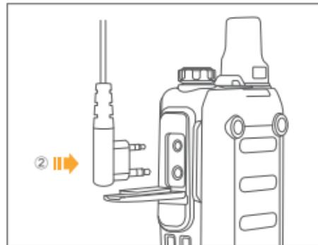
Open the jack cover and insert the earphone/programming cable into the radio. Keep covered if not in use.
