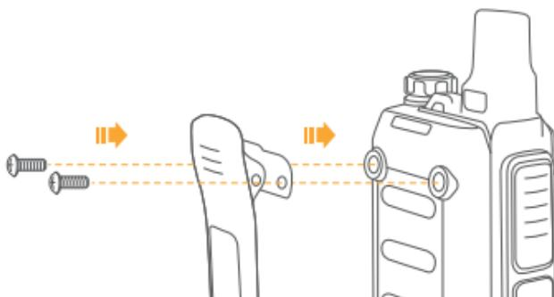
To install the belt clip, remove the screws from the back of the battery and install the belt clip.
