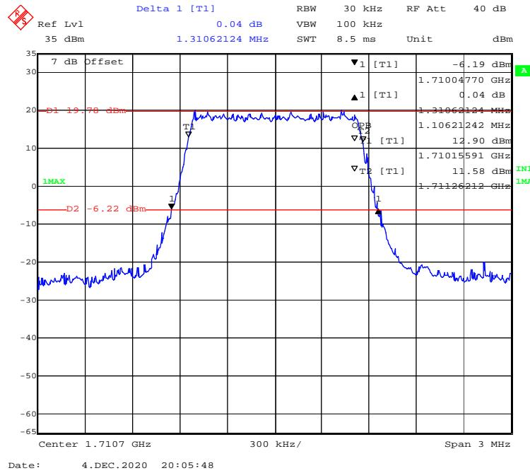
**16-QAM (3 MHz) - 99% Occupied & 26 dB Emissions Bandwidth, Low channel**
