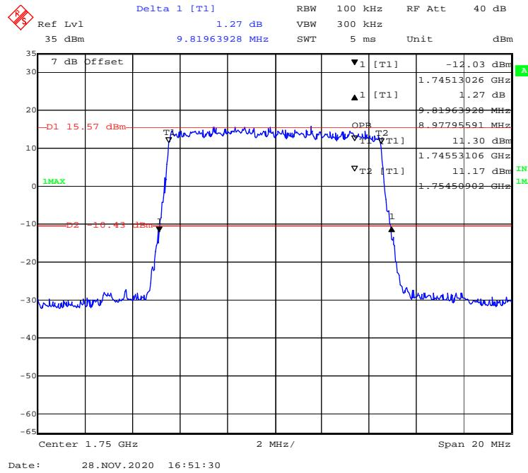
**QPSK (15 MHz) - 99% Occupied & 26 dB Emissions Bandwidth, High channel**
