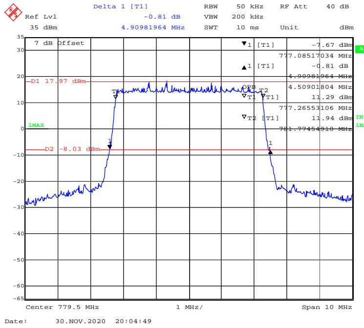
**QPSK (5 MHz) - 99% Occupied & 26 dB Emissions Bandwidth, Middle channel**
