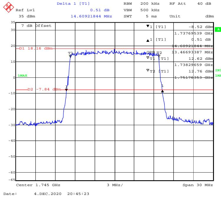
**16-QAM (20 MHz) - 99% Occupied & 26 dB Emissions Bandwidth, Middle channel**
