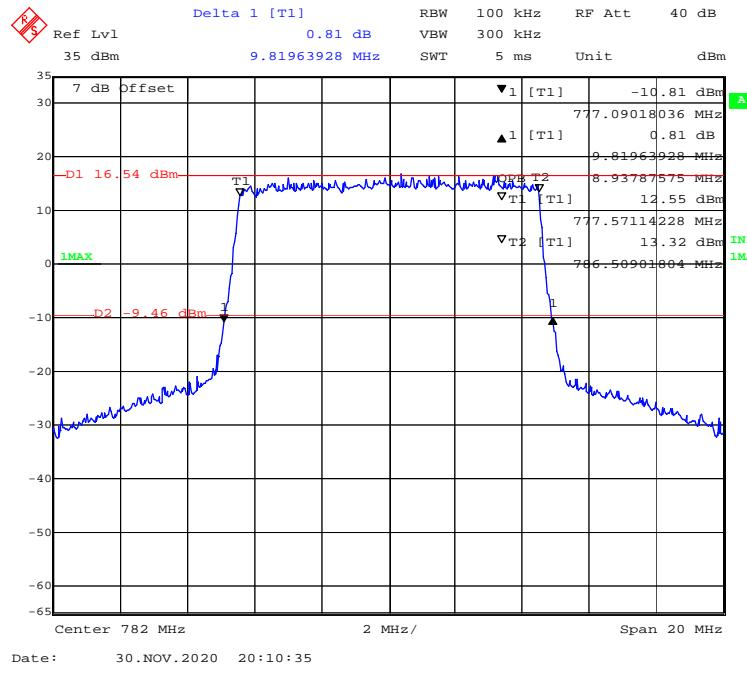
**16-QAM (5MHz) - 99% Occupied & 26 dB Emissions Bandwidth, Middle channel**
