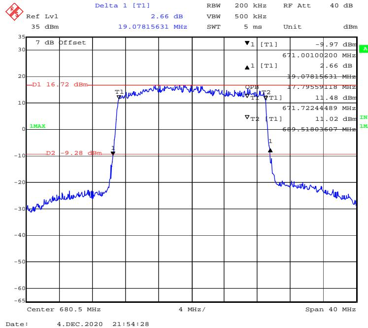
**16-QAM (5 MHz) - 99% Occupied & 26 dB Emissions Bandwidth, Middle channel**
