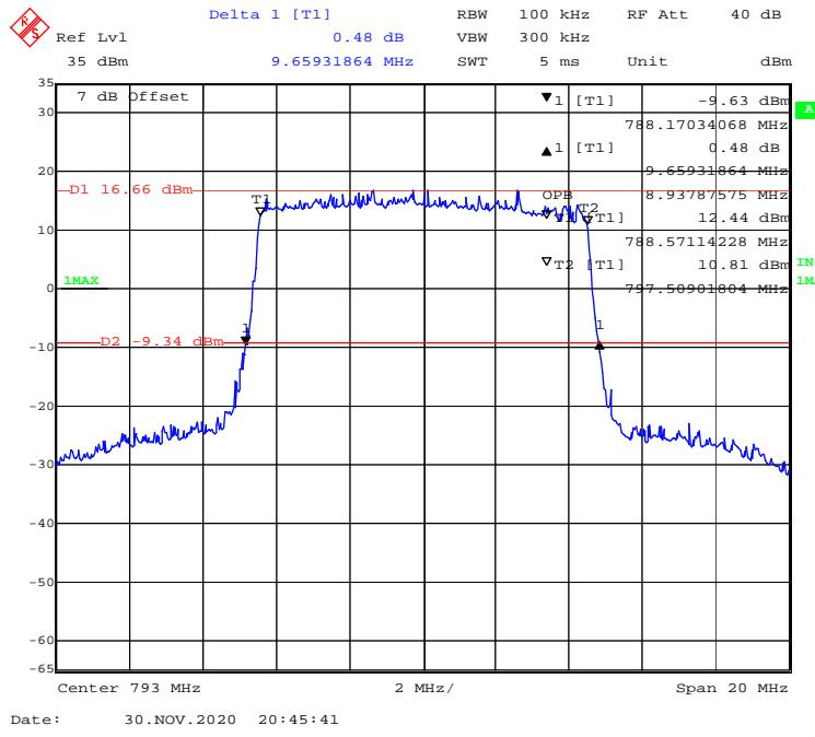
**16-QAM (5MHz) - 99% Occupied & 26 dB Emissions Bandwidth, Middle channel**
