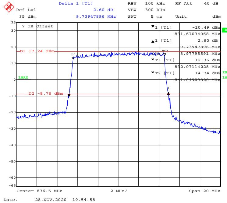
**16-QAM (1.4 MHz) - 99% Occupied & 26 dB Emissions Bandwidth, Middle channel**
