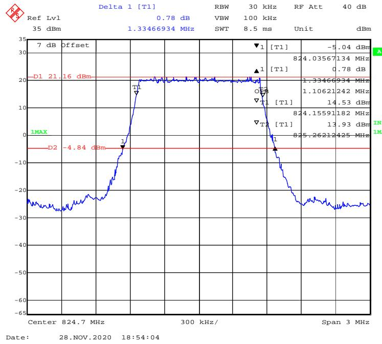
**QPSK (3.0 MHz) - 99% Occupied & 26 dB Emissions Bandwidth, Low channel**
