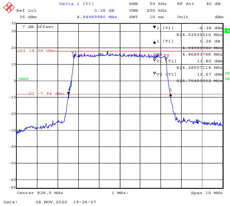
**16-QAM (10.0 MHz) - 99% Occupied & 26 dB Emissions Bandwidth, Low channel**
