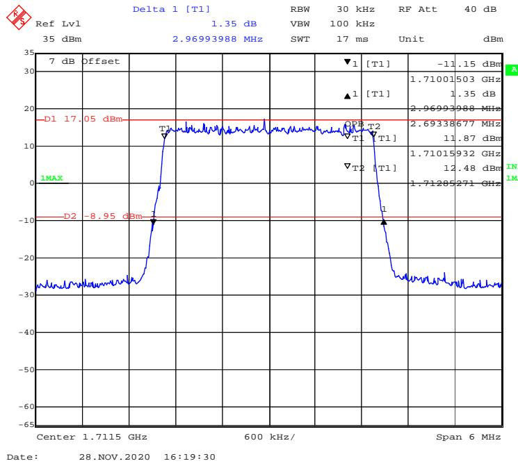
**QPSK (5MHz) - 99% Occupied & 26 dB Emissions Bandwidth, Low channel**
