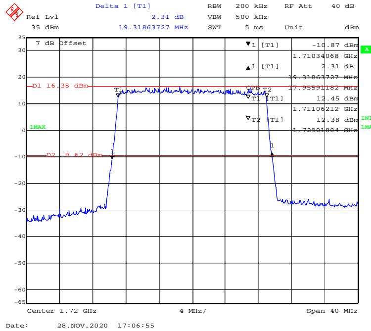
**16-QAM (1.4 MHz) - 99% Occupied & 26 dB Emissions Bandwidth, Low channel**
