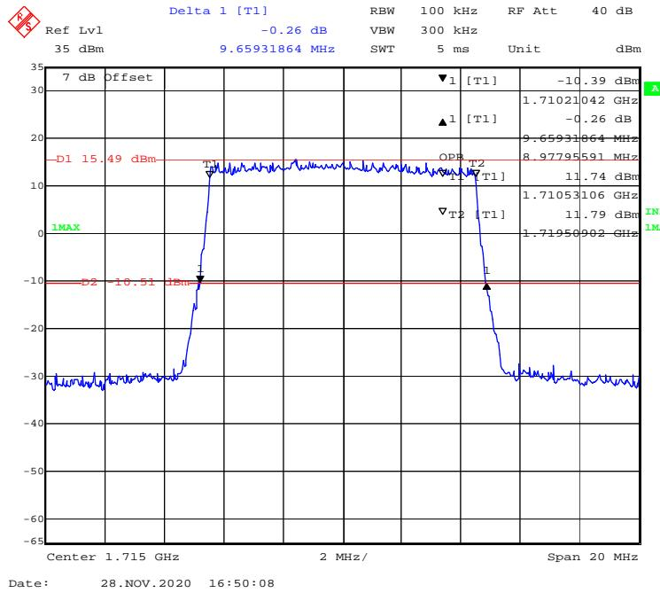
**16-QAM (15 MHz) - 99% Occupied & 26 dB Emissions Bandwidth, Low channel**
