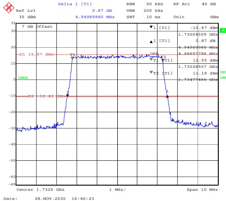
**16-QAM (10 MHz) - 99% Occupied & 26 dB Emissions Bandwidth, Middle channel**
