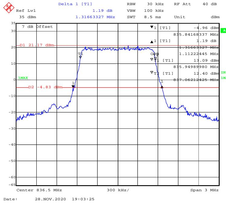
**QPSK (3.0 MHz) - 99% Occupied & 26 dB Emissions Bandwidth, Middle channel**
