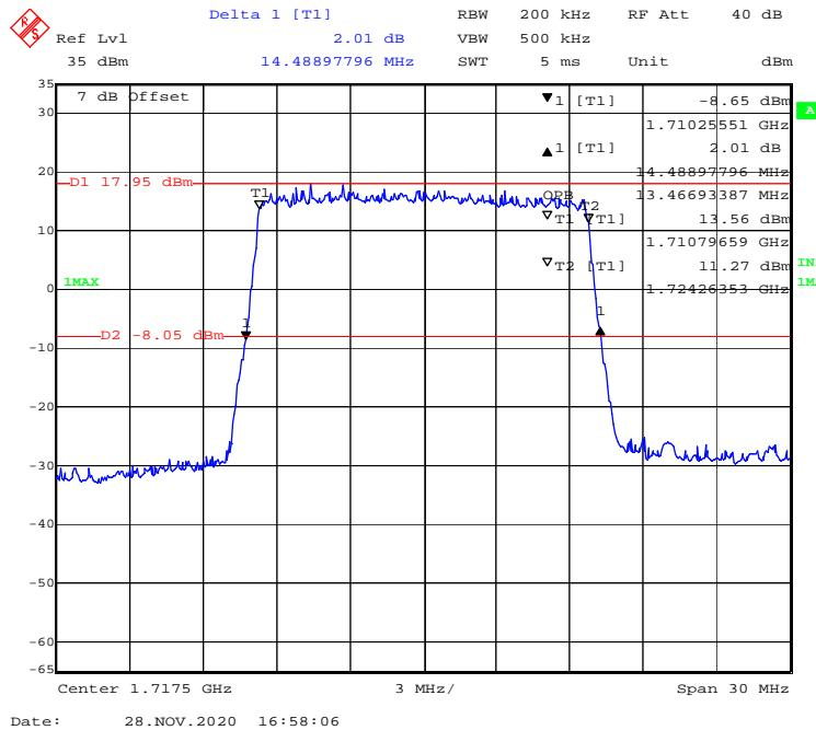
**16-QAM (20 MHz) - 99% Occupied & 26 dB Emissions Bandwidth, Low channel**
