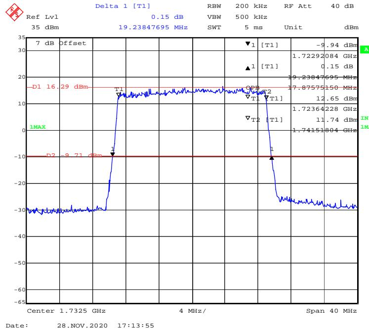
**16-QAM (1.4 MHz) - 99% Occupied & 26 dB Emissions Bandwidth, Middle channel**
