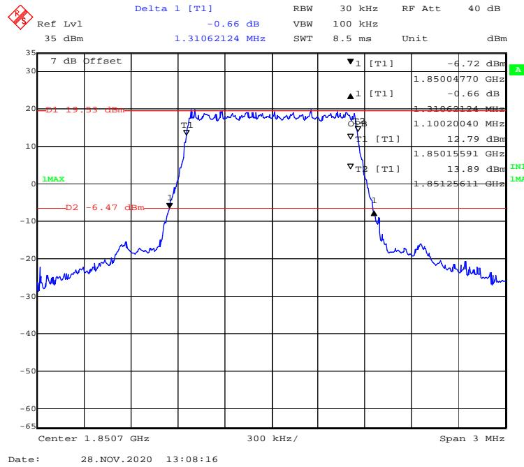
**16-QAM (3 MHz) - 99% Occupied & 26 dB Emissions Bandwidth, Low channel**
