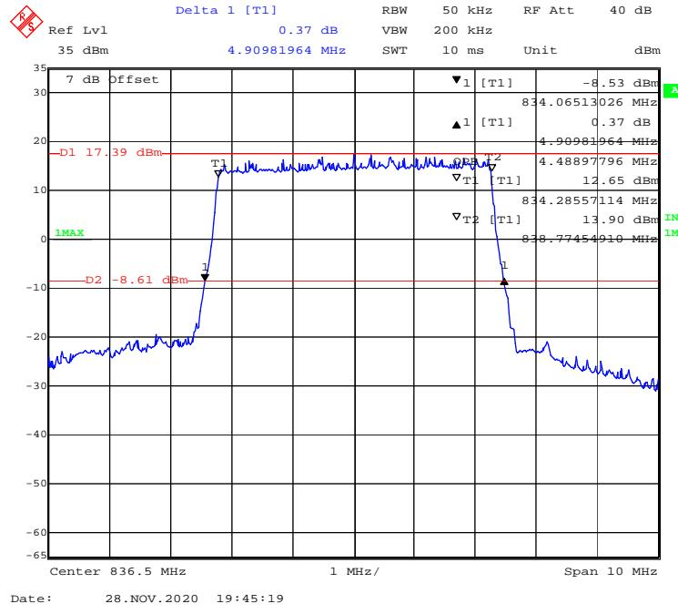
**QPSK (10.0 MHz) - 99% Occupied & 26 dB Emissions Bandwidth, Middle channel**
