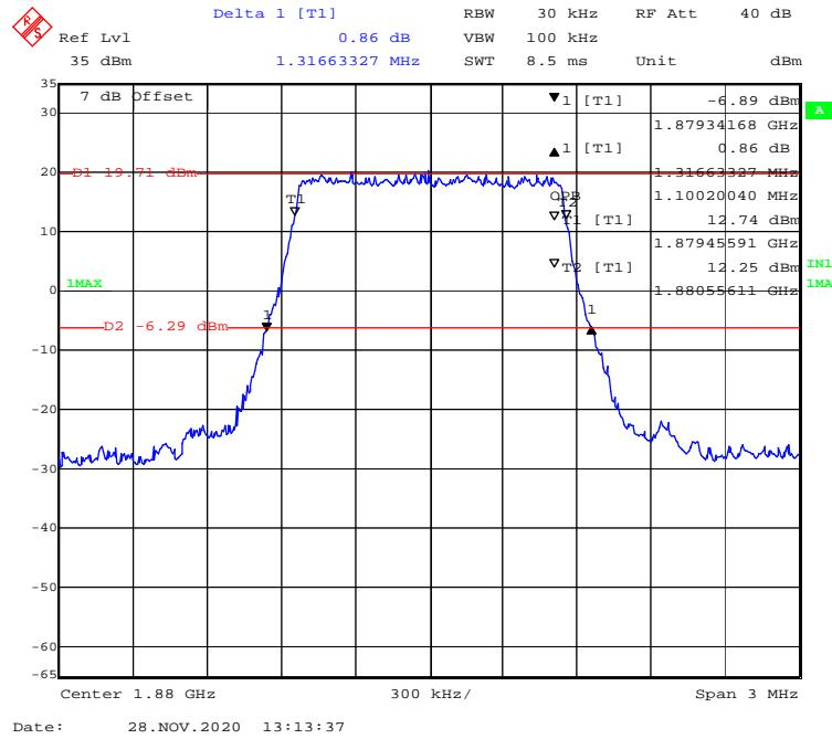
**QPSK (3 MHz) - 99% Occupied & 26 dB Emissions Bandwidth, Middle channel**
