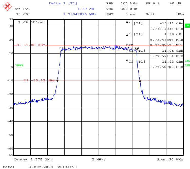
**QPSK (15 MHz) - 99% Occupied & 26 dB Emissions Bandwidth, High channel**
