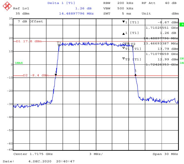
**QPSK (20 MHz) - 99% Occupied & 26 dB Emissions Bandwidth, Low channel**
