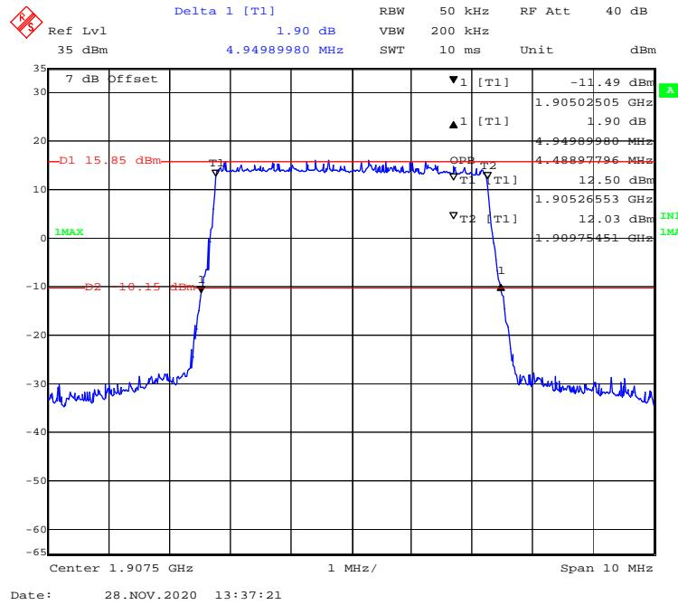
**QPSK (10MHz) - 99% Occupied & 26 dB Emissions Bandwidth, High channel**
