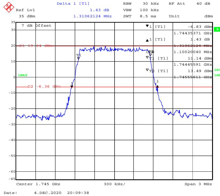
**16-QAM (3 MHz) - 99% Occupied & 26 dB Emissions Bandwidth, Middle channel**
