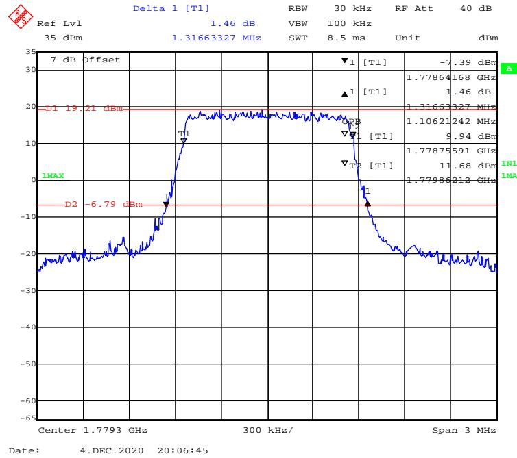
**QPSK (3 MHz) - 99% Occupied & 26 dB Emissions Bandwidth, High channel**
