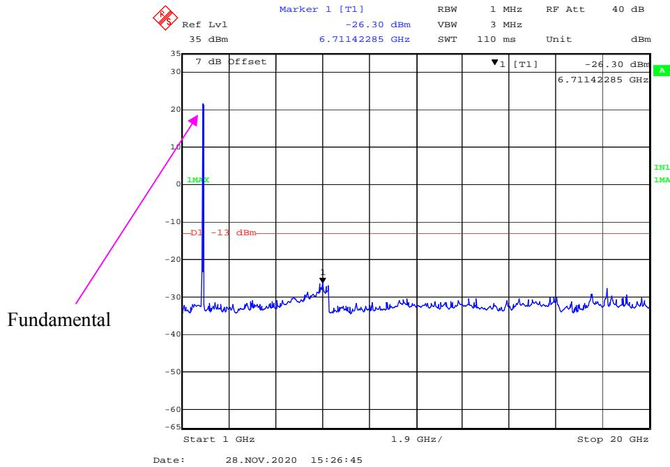
**30 MHz - 1 GHz (20 MHz, 16-QAM, Low Channel)**
