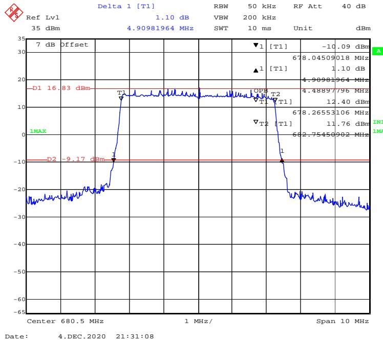
**QPSK (10MHz) - 99% Occupied & 26 dB Emissions Bandwidth, Middle channel**
