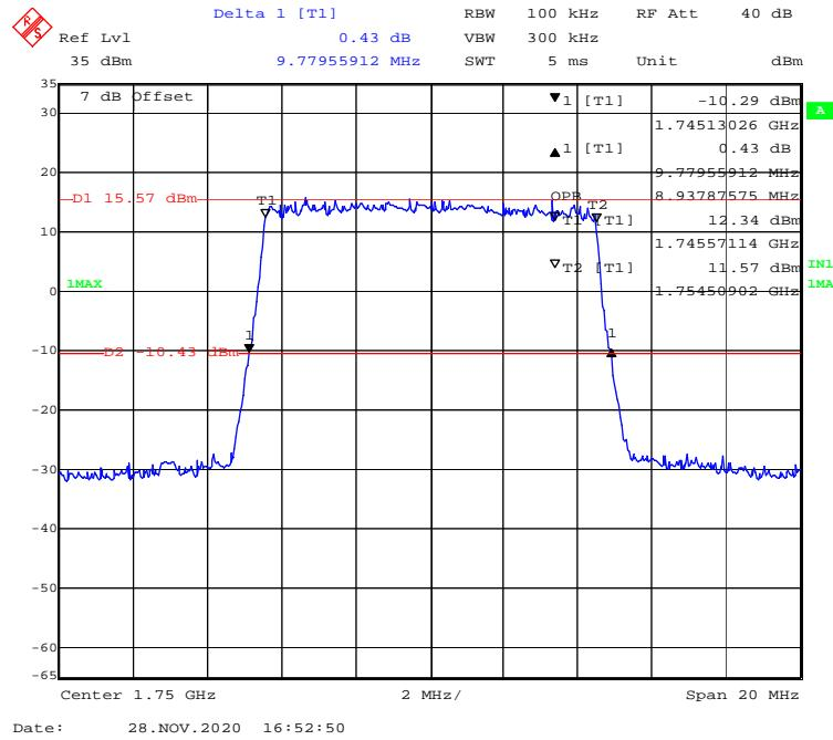
**16-QAM (15 MHz) - 99% Occupied & 26 dB Emissions Bandwidth, High channel**
