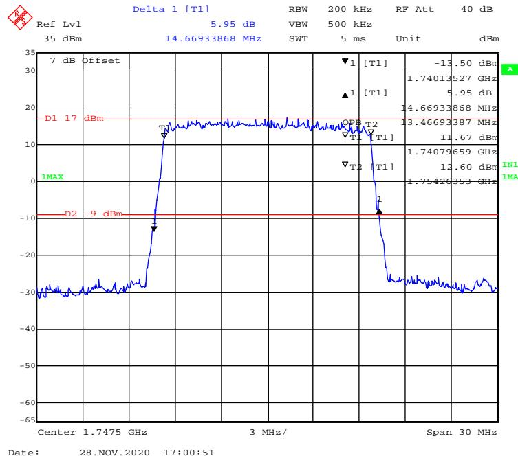
**16-QAM (20 MHz) - 99% Occupied & 26 dB Emissions Bandwidth, High channel**
