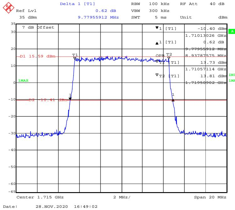
**QPSK (15 MHz) - 99% Occupied & 26 dB Emissions Bandwidth, Low channel**
