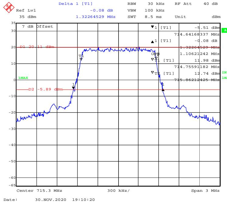
**16-QAM (3 MHz) - 99% Occupied & 26 dB Emissions Bandwidth, High channel**
