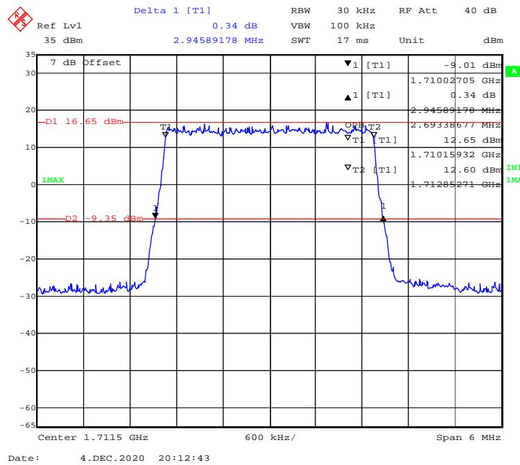
**QPSK (5 MHz) - 99% Occupied & 26 dB Emissions Bandwidth, Low channel**
