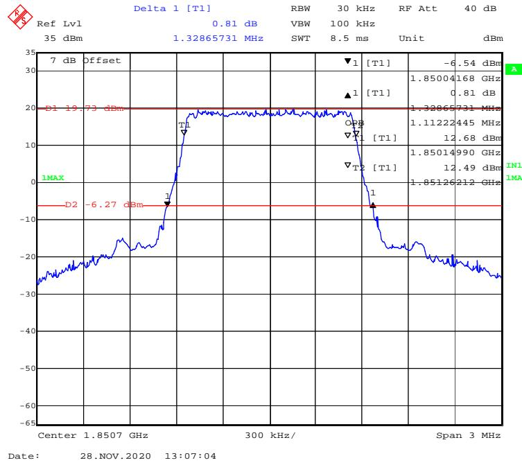
**QPSK (3 MHz) - 99% Occupied & 26 dB Emissions Bandwidth, Low channel**
