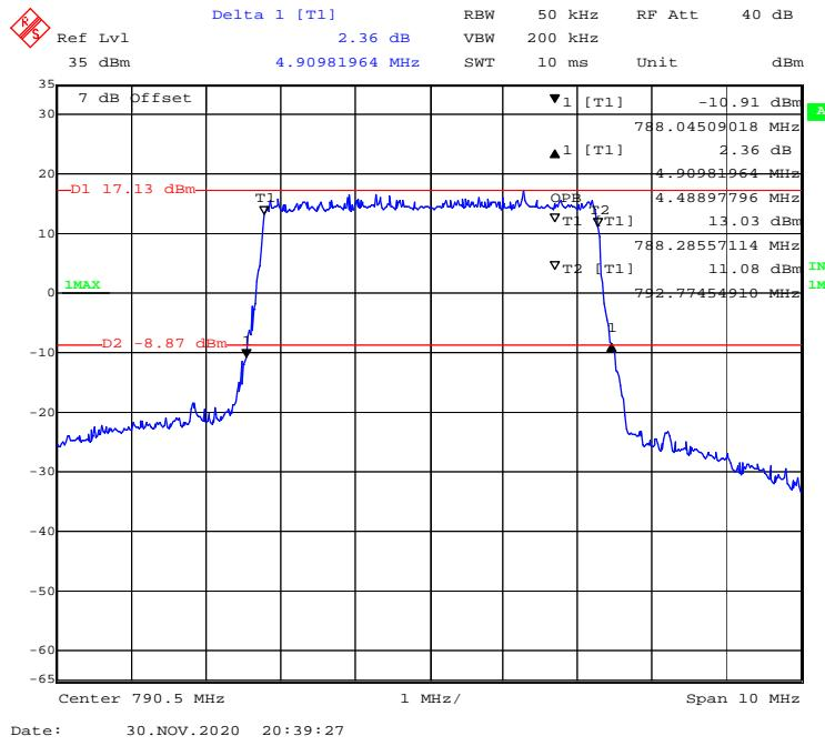
**QPSK (5 MHz) - 99% Occupied & 26 dB Emissions Bandwidth, Middle channel**
