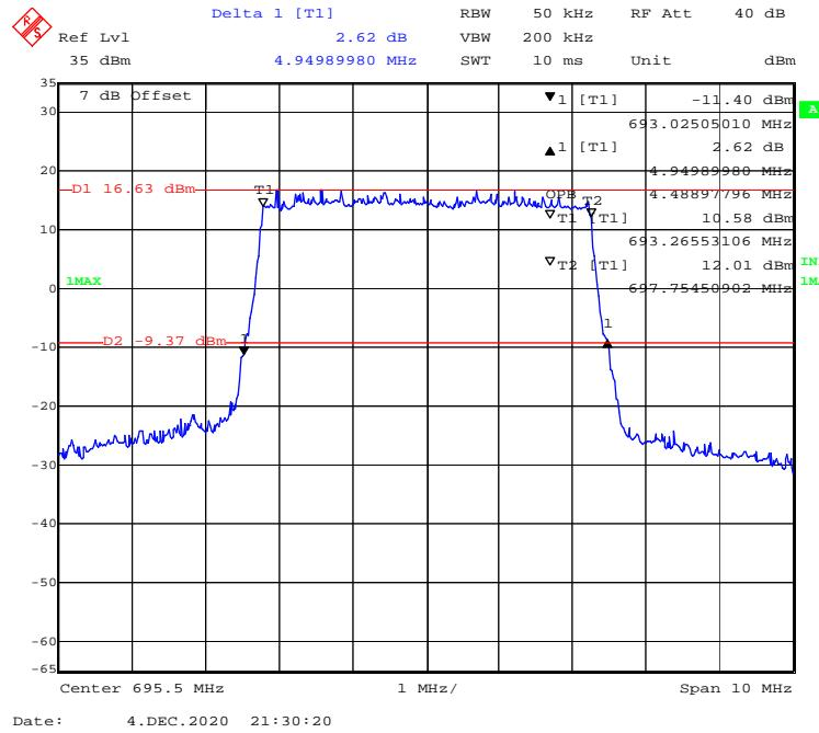
**16-QAM (10 MHz) - 99% Occupied & 26 dB Emissions Bandwidth, High channel**
