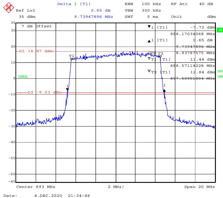
**QPSK (15 MHz) - 99% Occupied & 26 dB Emissions Bandwidth, High channel**
