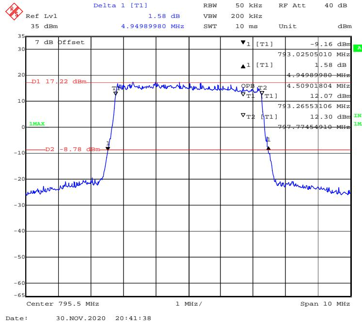
**16-QAM (5MHz) - 99% Occupied & 26 dB Emissions Bandwidth, High channel**
