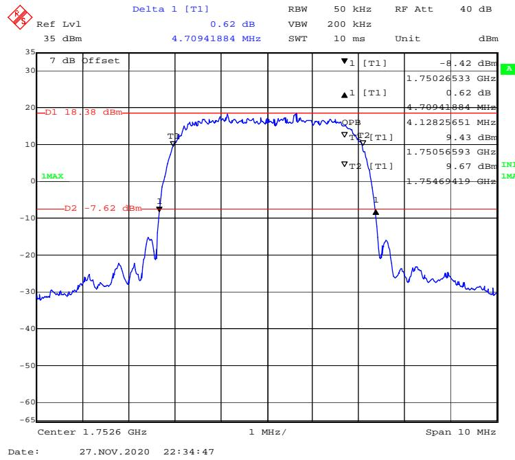
**99% Occupied & 26 dB Emissions Bandwidth for WCDMA (HSPA+) Mode, High Channel**
