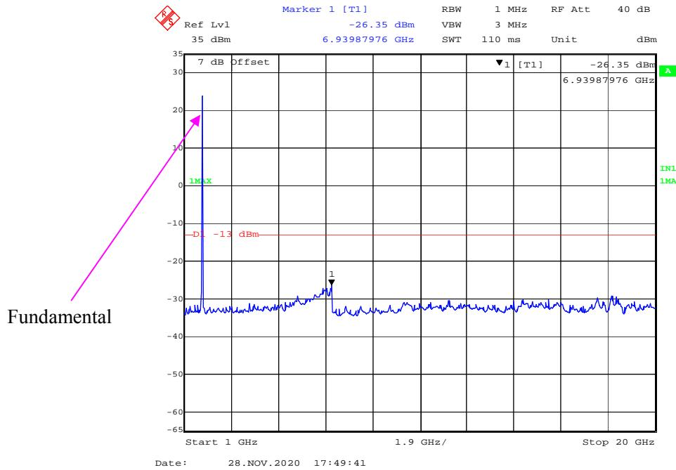
**30 MHz - 1 GHz (10 MHz, QPSK, Middle Channel)**
