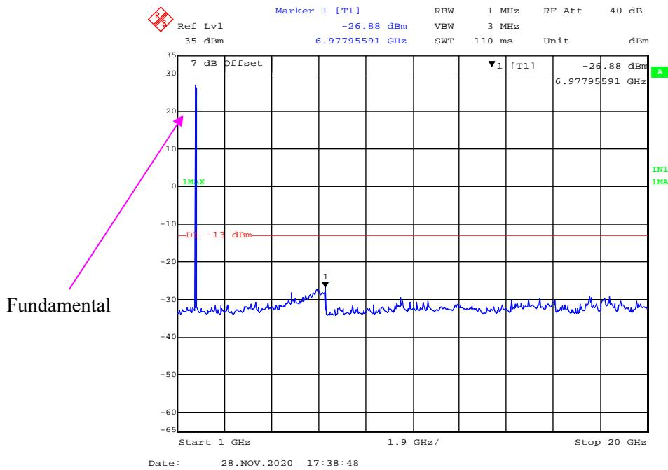
**30 MHz - 1 GHz (3 MHz, QPSK, High Channel)**
