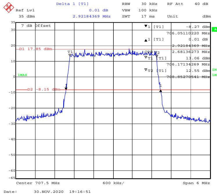
**16-QAM (5 MHz) - 99% Occupied & 26 dB Emissions Bandwidth, Middle channel**
