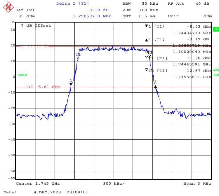
**QPSK (3 MHz) - 99% Occupied & 26 dB Emissions Bandwidth, Middle channel**
