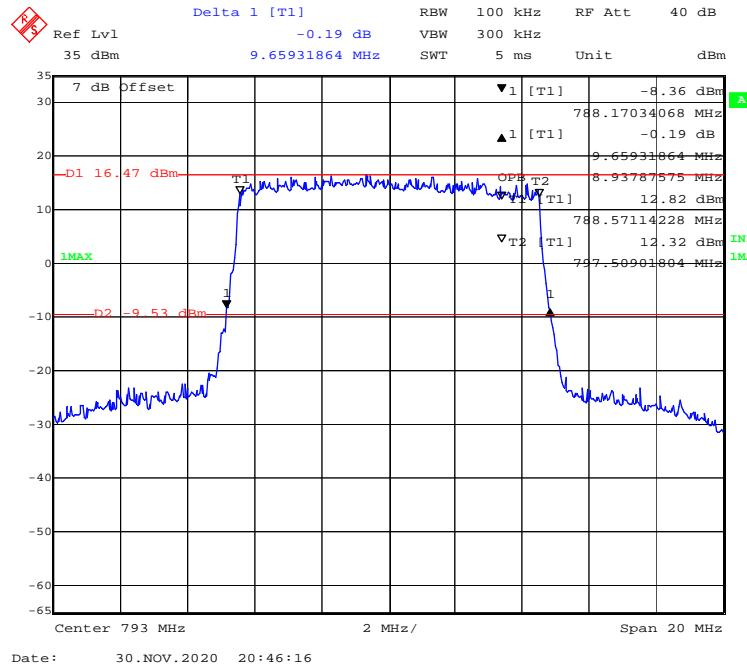
**QPSK (5 MHz) - 99% Occupied & 26 dB Emissions Bandwidth, High channel**
