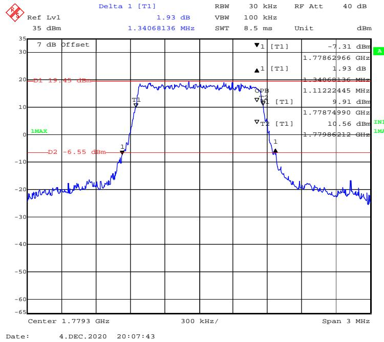
**16-QAM (3 MHz) - 99% Occupied & 26 dB Emissions Bandwidth, High channel**
