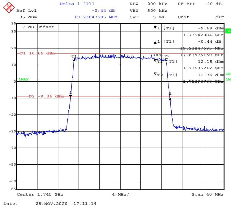
**16-QAM (1.4 MHz) - 99% Occupied & 26 dB Emissions Bandwidth, High channel**
