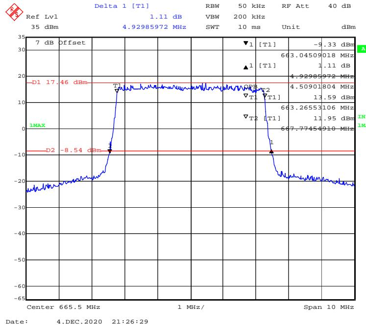
**QPSK (10MHz) - 99% Occupied & 26 dB Emissions Bandwidth, Low channel**
