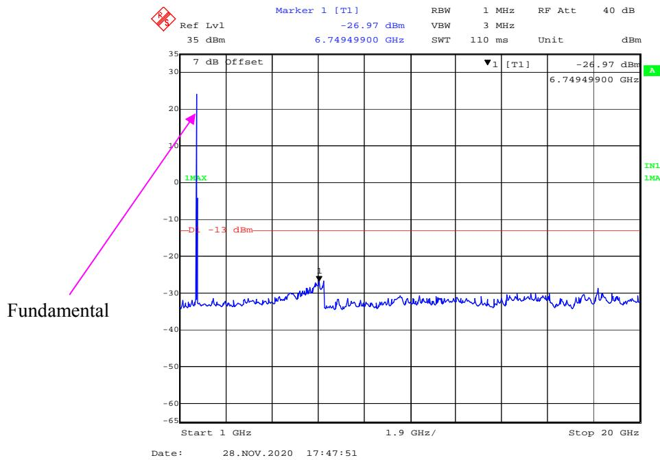
**30 MHz - 1 GHz (10 MHz, QPSK, Low Channel)**
