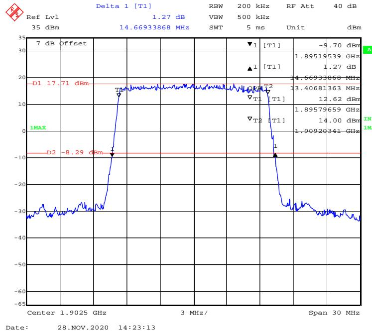
**QPSK (20 MHz) - 99% Occupied & 26 dB Emissions Bandwidth, High channel**
