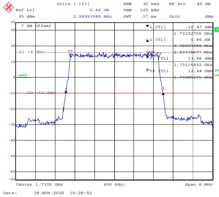
**QPSK (5MHz) - 99% Occupied & 26 dB Emissions Bandwidth, Middle channel**
