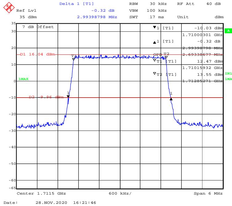
**16-QAM (5 MHz) - 99% Occupied & 26 dB Emissions Bandwidth, Low channel**
