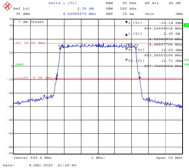
**QPSK (10MHz) - 99% Occupied & 26 dB Emissions Bandwidth, High channel**
