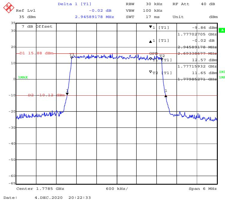
**16-QAM (5 MHz) - 99% Occupied & 26 dB Emissions Bandwidth, High channel**
