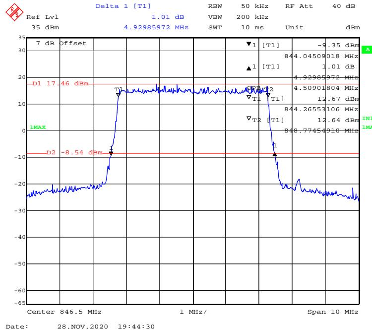
**16-QAM (10.0 MHz) - 99% Occupied & 26 dB Emissions Bandwidth, High channel**
