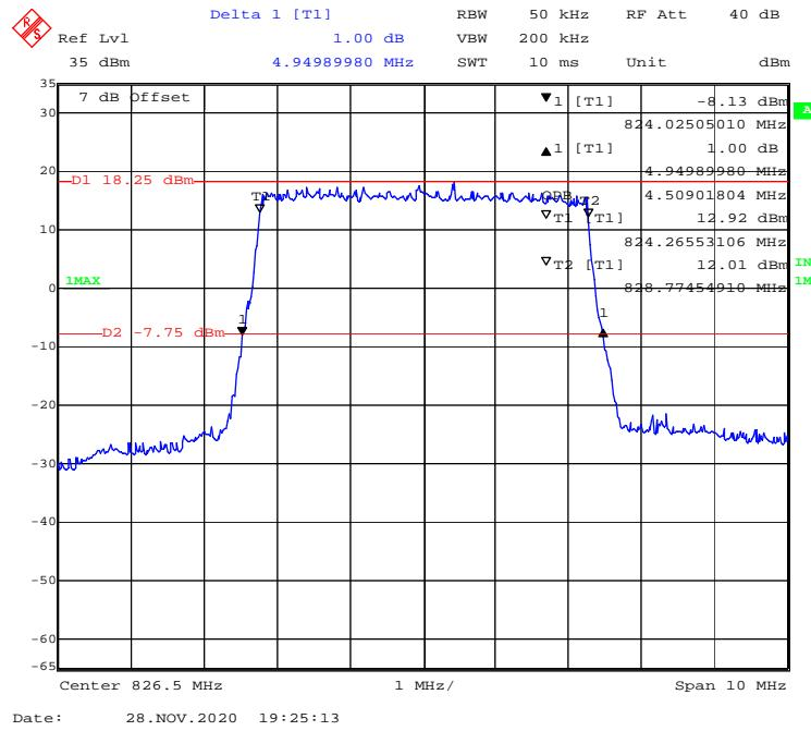
**QPSK (10.0 MHz) - 99% Occupied & 26 dB Emissions Bandwidth, Low channel**
