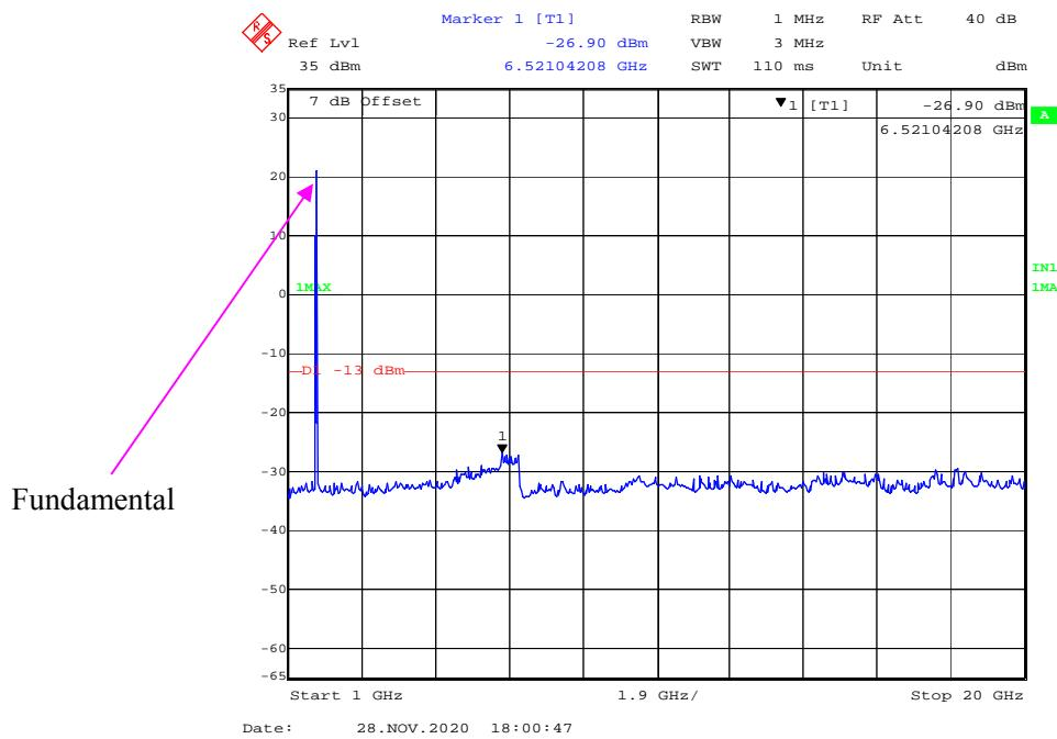
**30 MHz - 1 GHz (1.4 MHz, QPSK, High Channel)**
