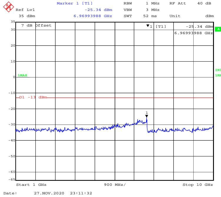
**WCDMA Band II:****30 MHz – 1GHz WCDMA (Rel 99) Mode, Low channel**
