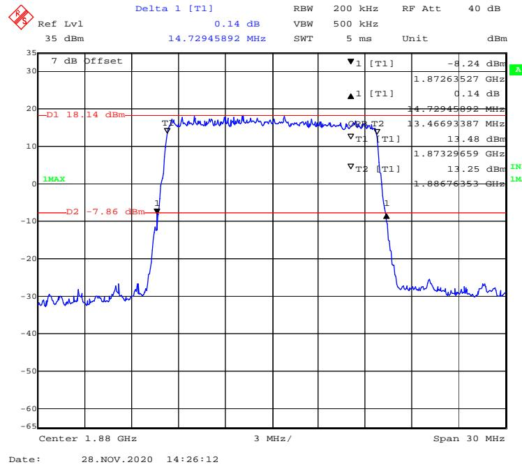
**QPSK (20 MHz) - 99% Occupied & 26 dB Emissions Bandwidth, Middle channel**
