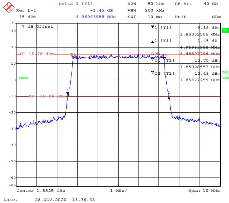
**16-QAM (10 MHz) - 99% Occupied & 26 dB Emissions Bandwidth, Low channel**
