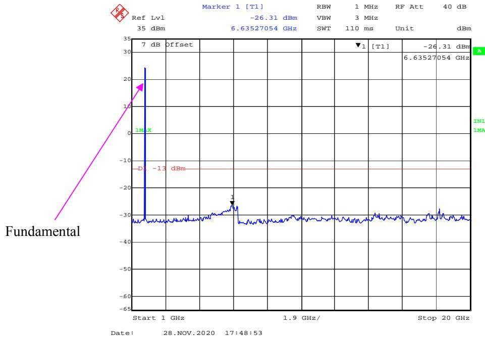
**30 MHz - 1 GHz (5 MHz, 16-QAM, High Channel)**
