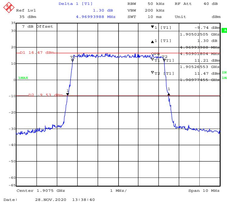
**16-QAM (10 MHz) - 99% Occupied & 26 dB Emissions Bandwidth, High channel**
