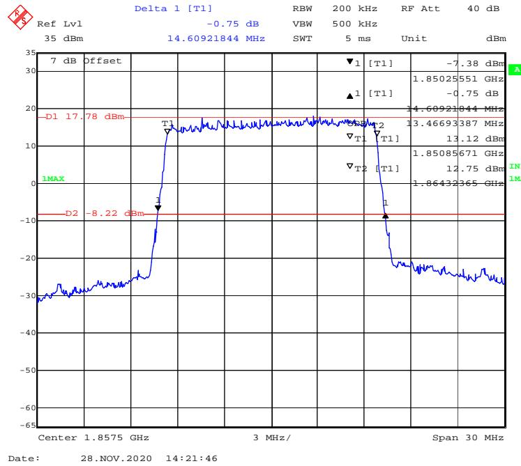
**16-QAM (20 MHz) - 99% Occupied & 26 dB Emissions Bandwidth, Low channel**
