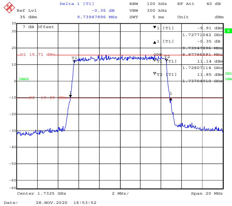
**QPSK (15 MHz) - 99% Occupied & 26 dB Emissions Bandwidth, Middle channel**
