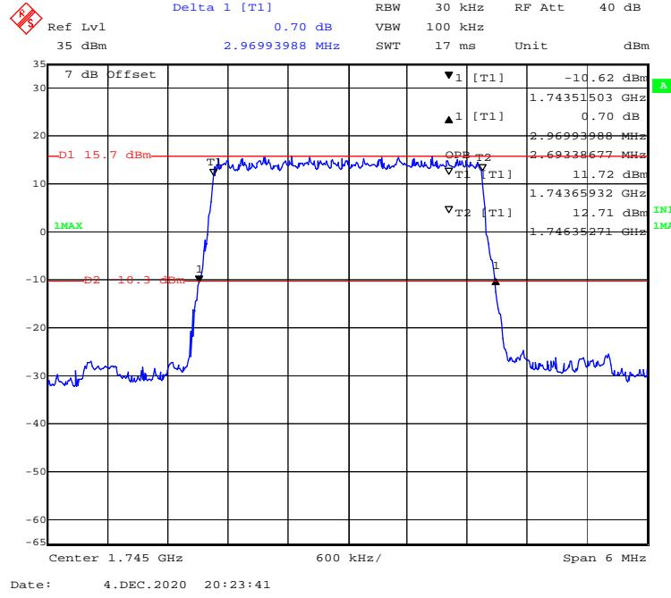
**QPSK (5 MHz) - 99% Occupied & 26 dB Emissions Bandwidth, Middle channel**
