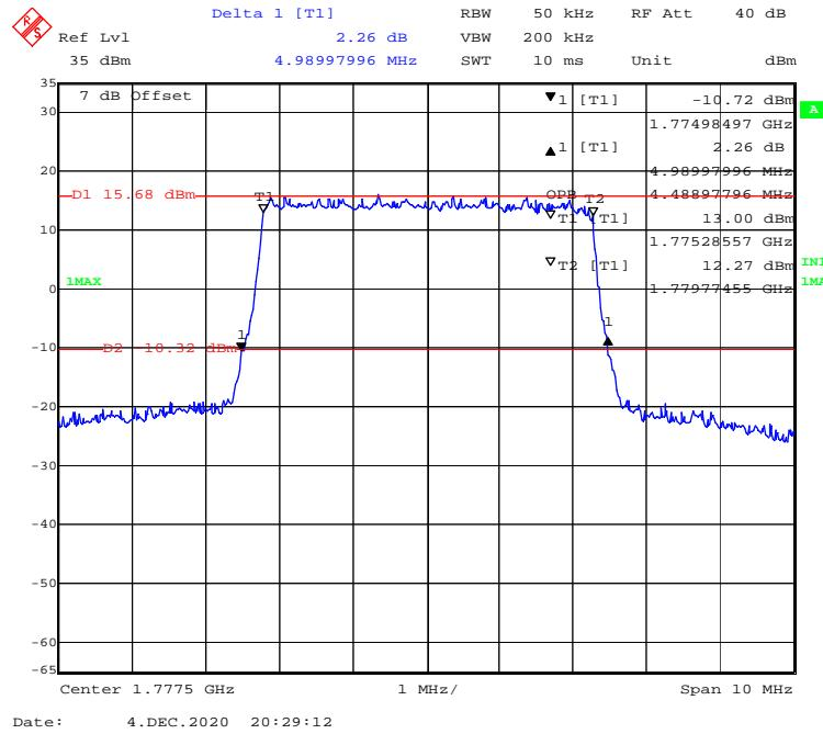
**QPSK (10MHz) - 99% Occupied & 26 dB Emissions Bandwidth, High channel**
