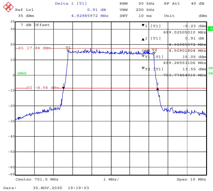
**16-QAM (10 MHz) - 99% Occupied & 26 dB Emissions Bandwidth, Low channel**
