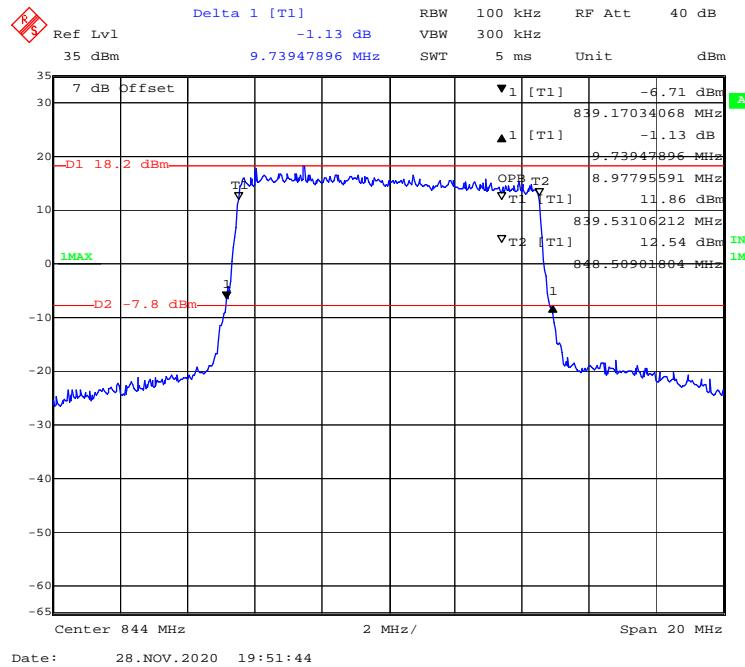
**16-QAM (1.4 MHz) - 99% Occupied & 26 dB Emissions Bandwidth, High channel**
