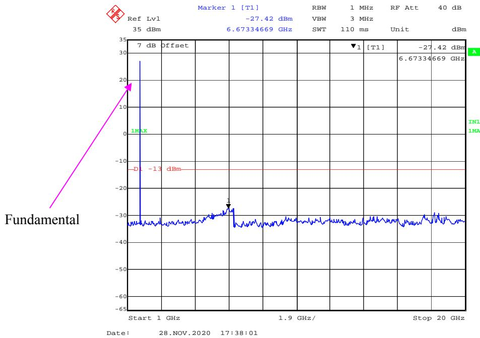
**30 MHz - 1 GHz (3 MHz, QPSK, Low Channel)**
