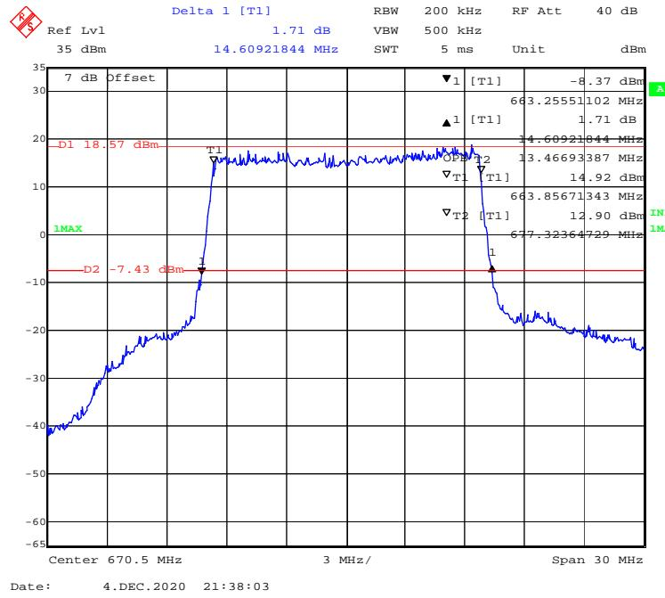
**QPSK (20 MHz) - 99% Occupied & 26 dB Emissions Bandwidth, Low channel**
