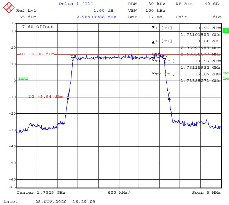
**16-QAM (5 MHz) - 99% Occupied & 26 dB Emissions Bandwidth, Middle channel**
