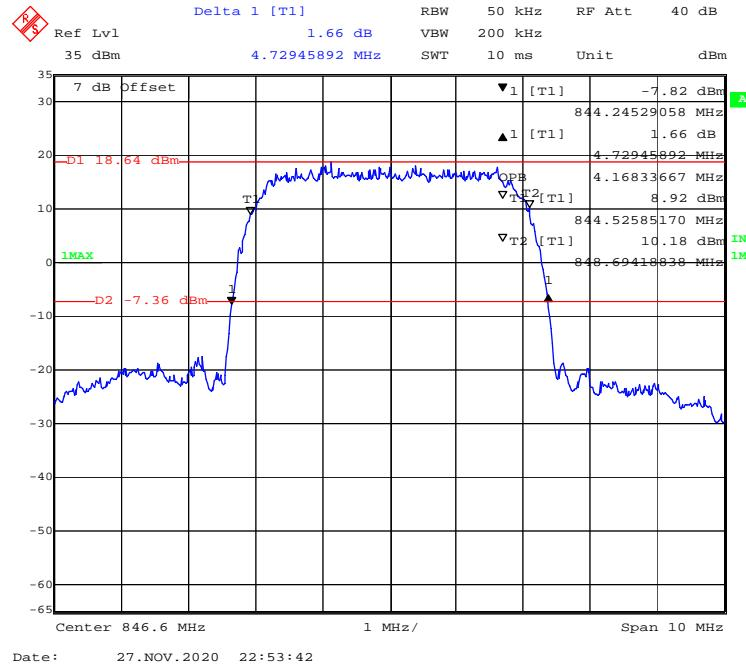
**99% Occupied & 26 dB Emissions Bandwidth for WCDMA (HSDPA) Mode, High Channel**
