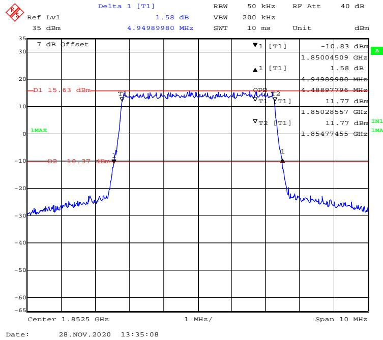
**QPSK (10MHz) - 99% Occupied & 26 dB Emissions Bandwidth, Low channel**
