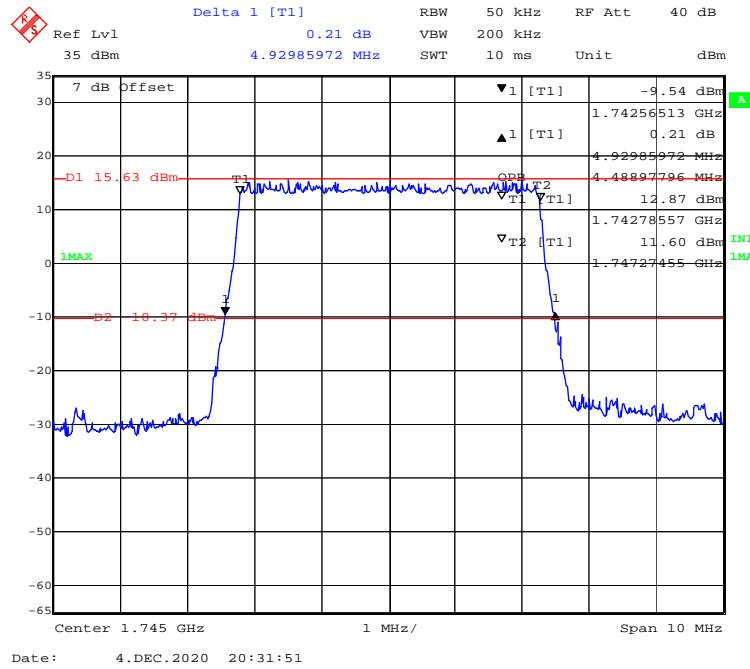
**16-QAM (10 MHz) - 99% Occupied & 26 dB Emissions Bandwidth, Middle channel**
