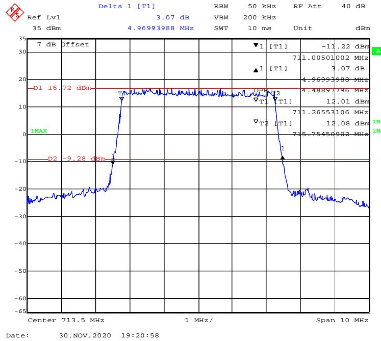
**16-QAM (10 MHz) - 99% Occupied & 26 dB Emissions Bandwidth, High channel**
