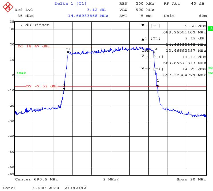
**16-QAM (20 MHz) - 99% Occupied & 26 dB Emissions Bandwidth, High channel**
