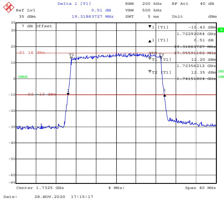
**QPSK (1.4 MHz) - 99% Occupied & 26 dB Emissions Bandwidth, High channel**
