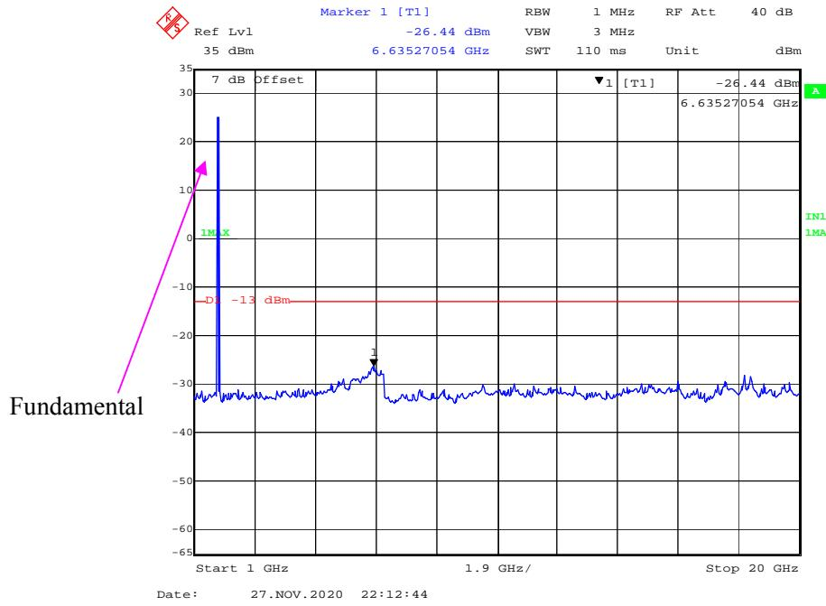
**LTE Band 2:****30 MHz - 1 GHz (1.4 MHz, QPSK, Low Channel)**
