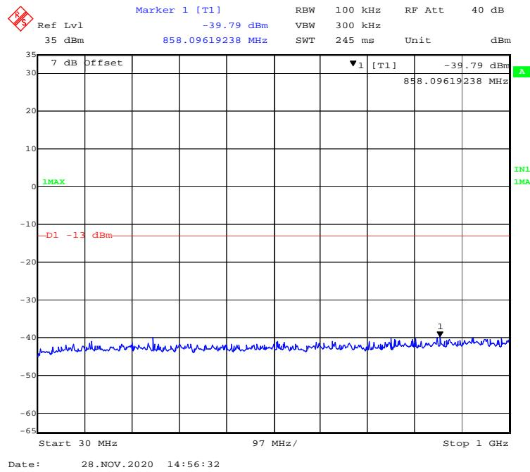
**1 GHz – 20 GHz (5 MHz, 16-QAM, Middle Channel)**
