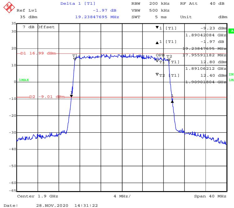
**16-QAM (1.4 MHz) - 99% Occupied & 26 dB Emissions Bandwidth, High channel**
