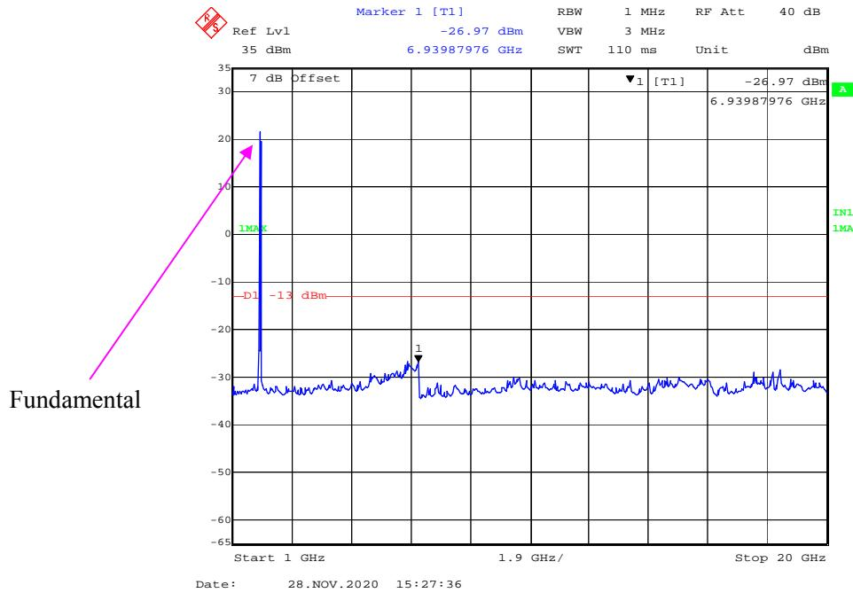
**LTE Band 4:****30 MHz - 1 GHz (1.4 MHz, QPSK, Low Channel)**
