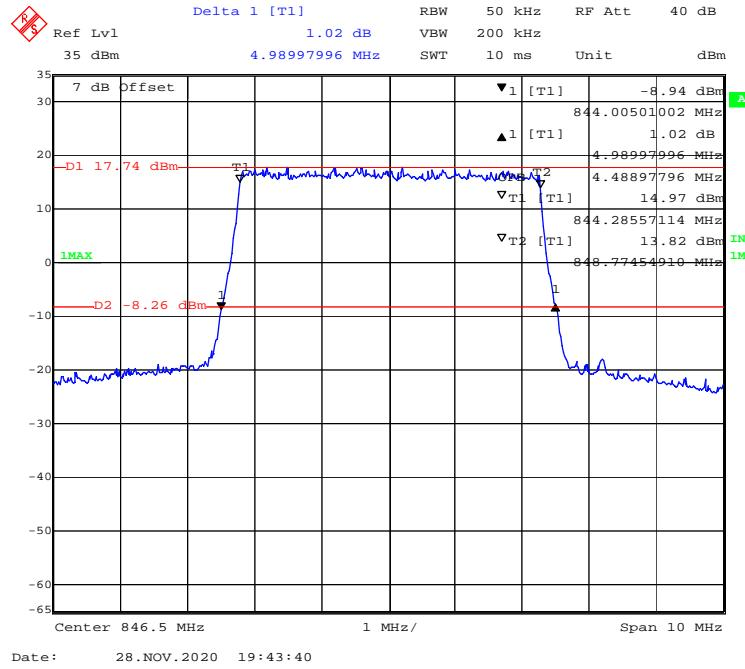
**QPSK (10.0 MHz) - 99% Occupied & 26 dB Emissions Bandwidth, High channel**
