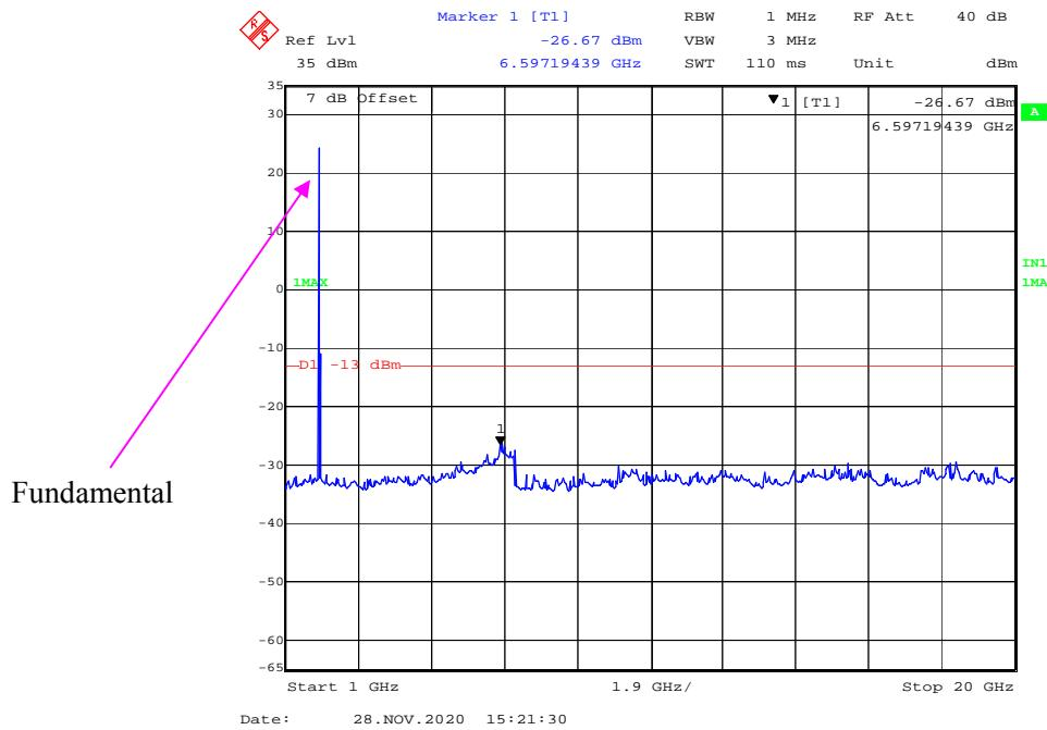
**30 MHz - 1 GHz (10 MHz, QPSK, High Channel)**
