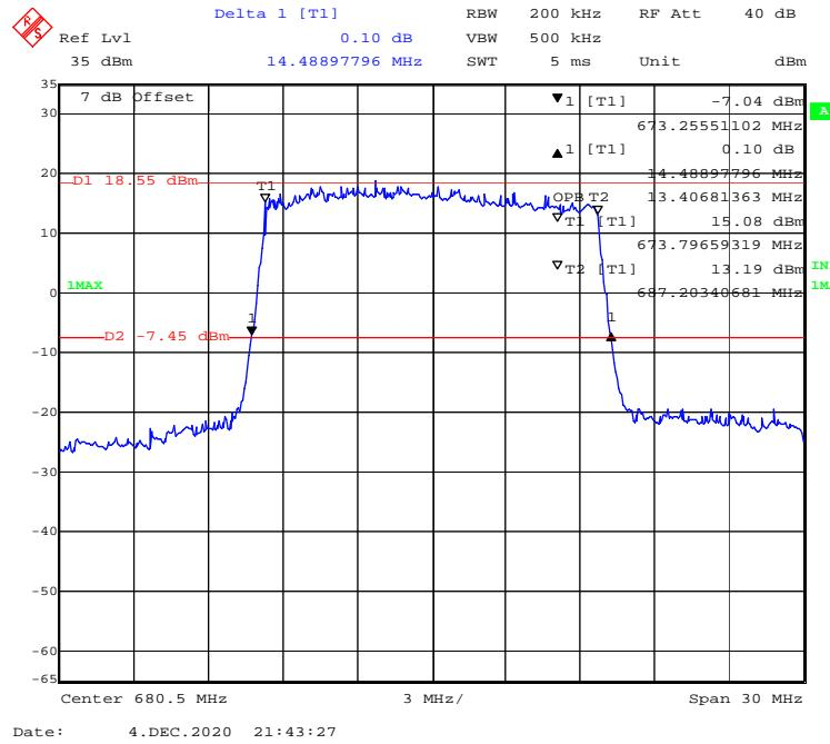
**QPSK (20 MHz) - 99% Occupied & 26 dB Emissions Bandwidth, Middle channel**
