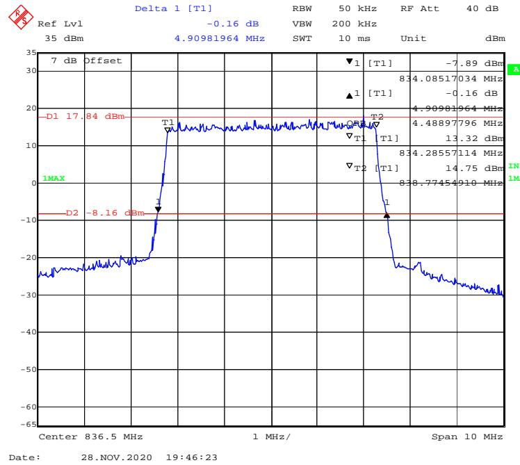
**16-QAM (10.0 MHz) - 99% Occupied & 26 dB Emissions Bandwidth, Middle channel**
