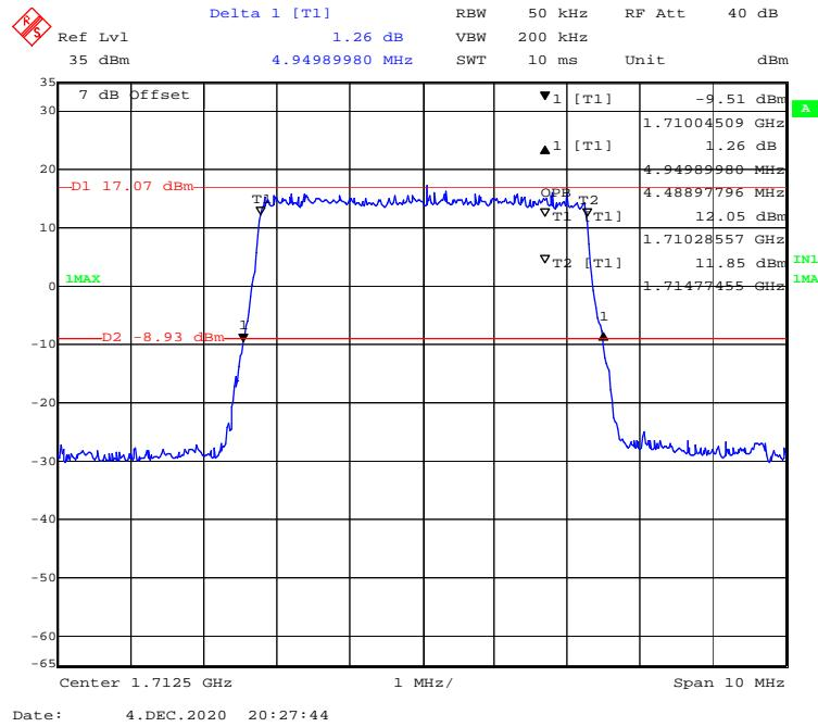
**16-QAM (10 MHz) - 99% Occupied & 26 dB Emissions Bandwidth, Low channel**
