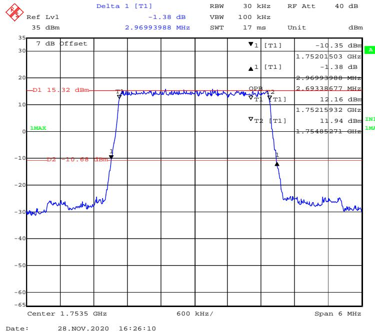
**16-QAM (5 MHz) - 99% Occupied & 26 dB Emissions Bandwidth, High channel**
