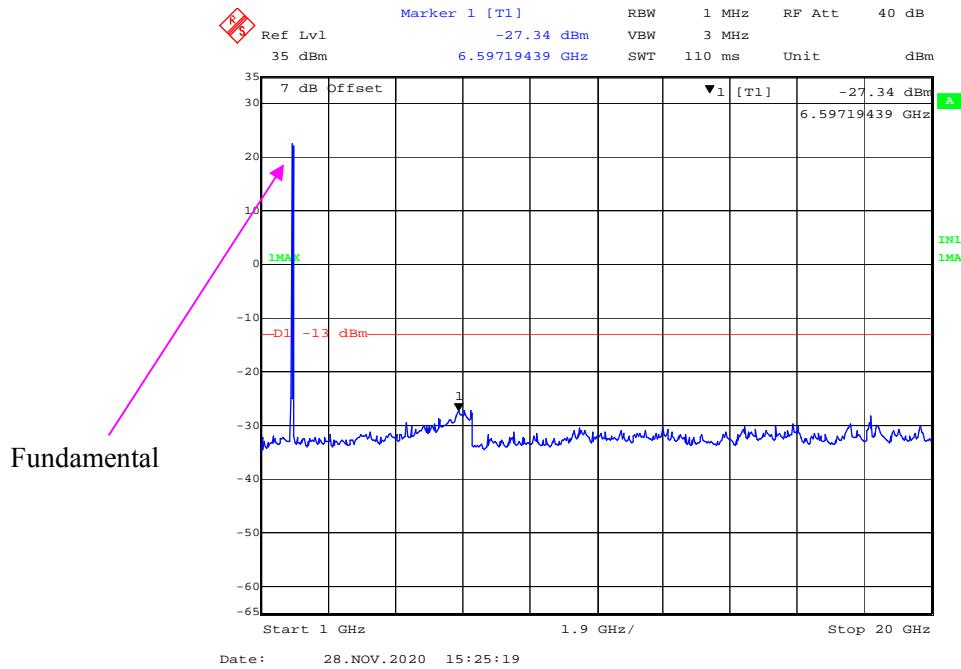
**30 MHz - 1 GHz (15 MHz, 16-QAM, High Channel)**
