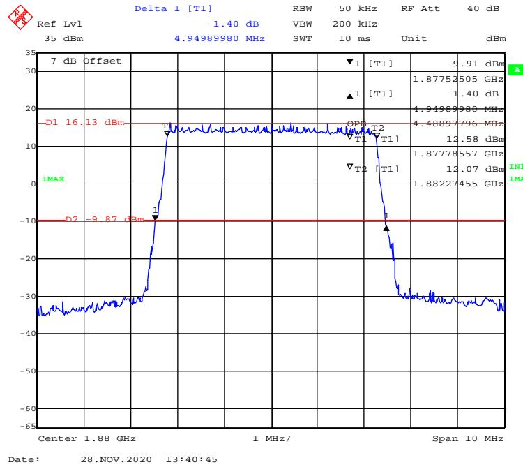
**16-QAM (10 MHz) - 99% Occupied & 26 dB Emissions Bandwidth, Middle channel**
