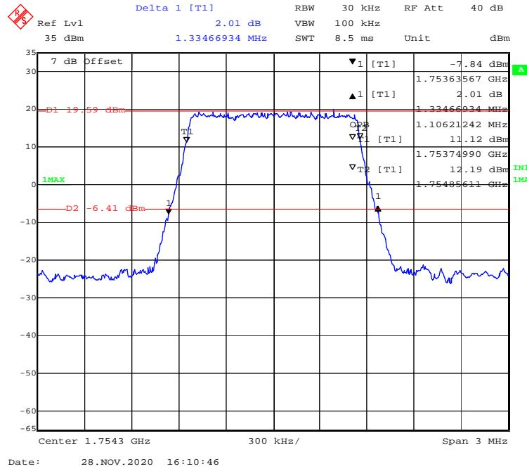
**QPSK (3 MHz) - 99% Occupied & 26 dB Emissions Bandwidth, High channel**
