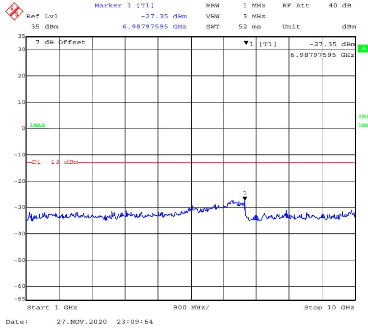
**30 MHz – 1GHz WCDMA (HSDPA) Mode, Middle channel**
