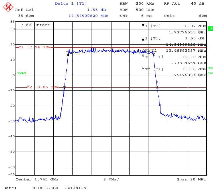
**QPSK (20 MHz) - 99% Occupied & 26 dB Emissions Bandwidth, Middle channel**
