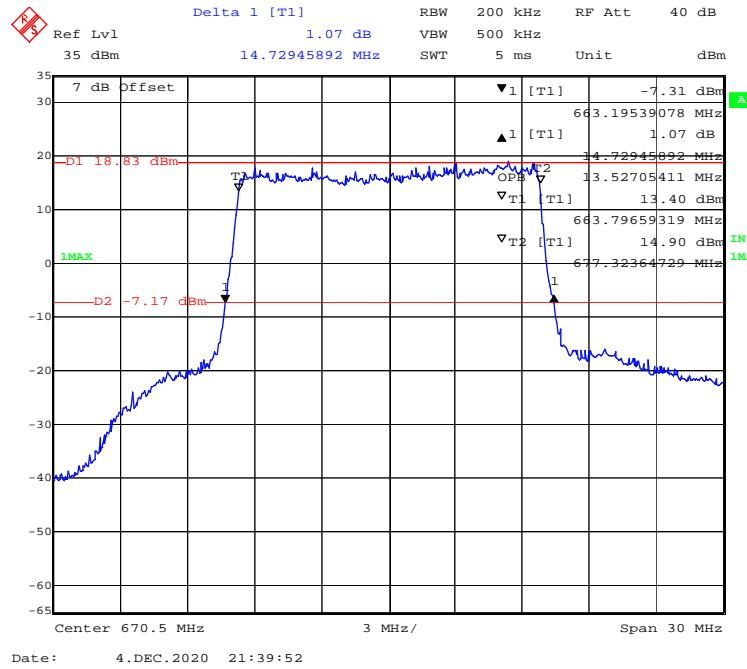
**16-QAM (20 MHz) - 99% Occupied & 26 dB Emissions Bandwidth, Low channel**
