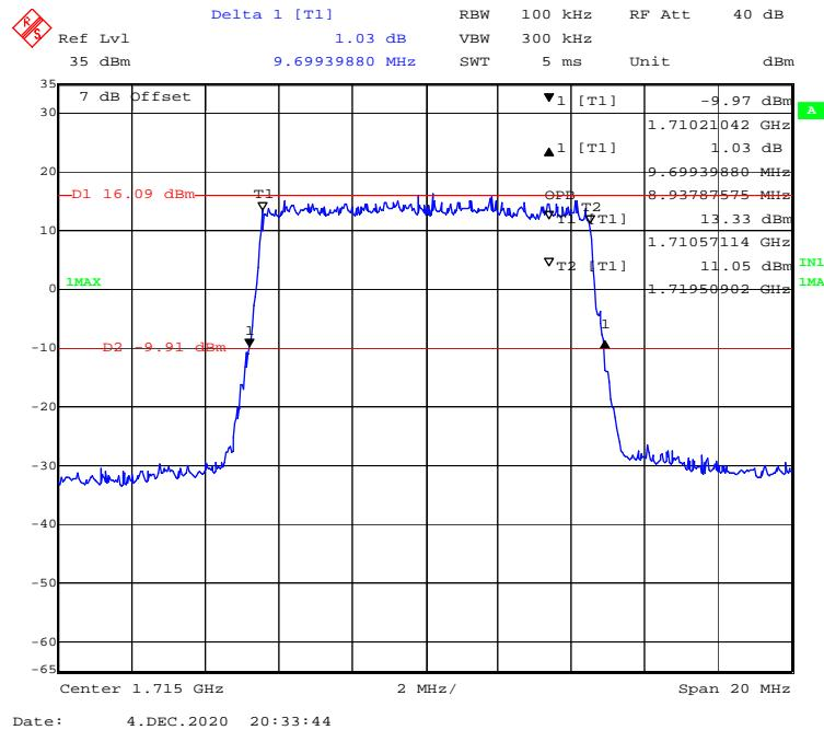
**16-QAM (15 MHz) - 99% Occupied & 26 dB Emissions Bandwidth, Low channel**
