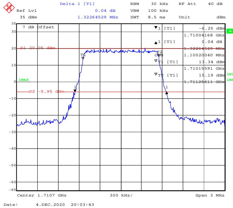
**QPSK (3 MHz) - 99% Occupied & 26 dB Emissions Bandwidth, Low channel**
