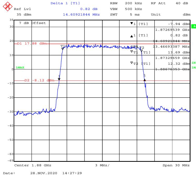
**16-QAM (20 MHz) - 99% Occupied & 26 dB Emissions Bandwidth, Middle channel**
