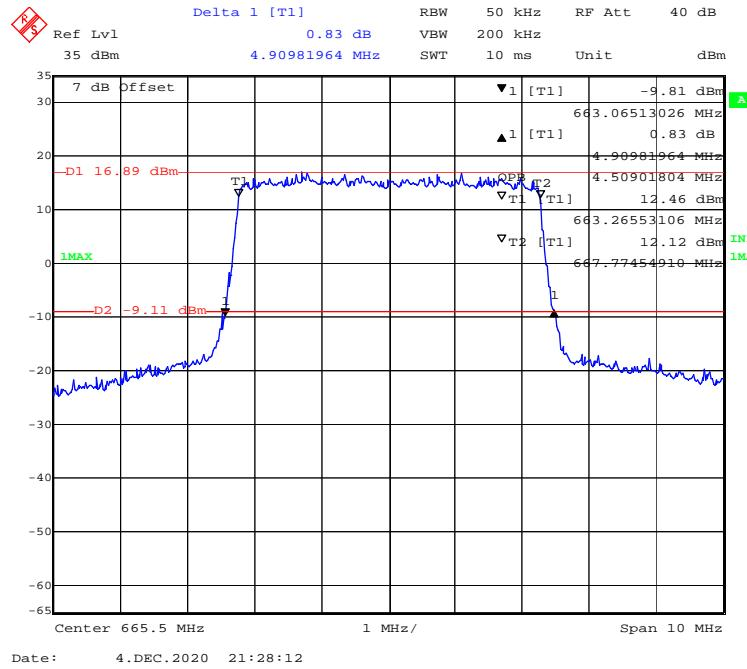
**16-QAM (10 MHz) - 99% Occupied & 26 dB Emissions Bandwidth, Low channel**
