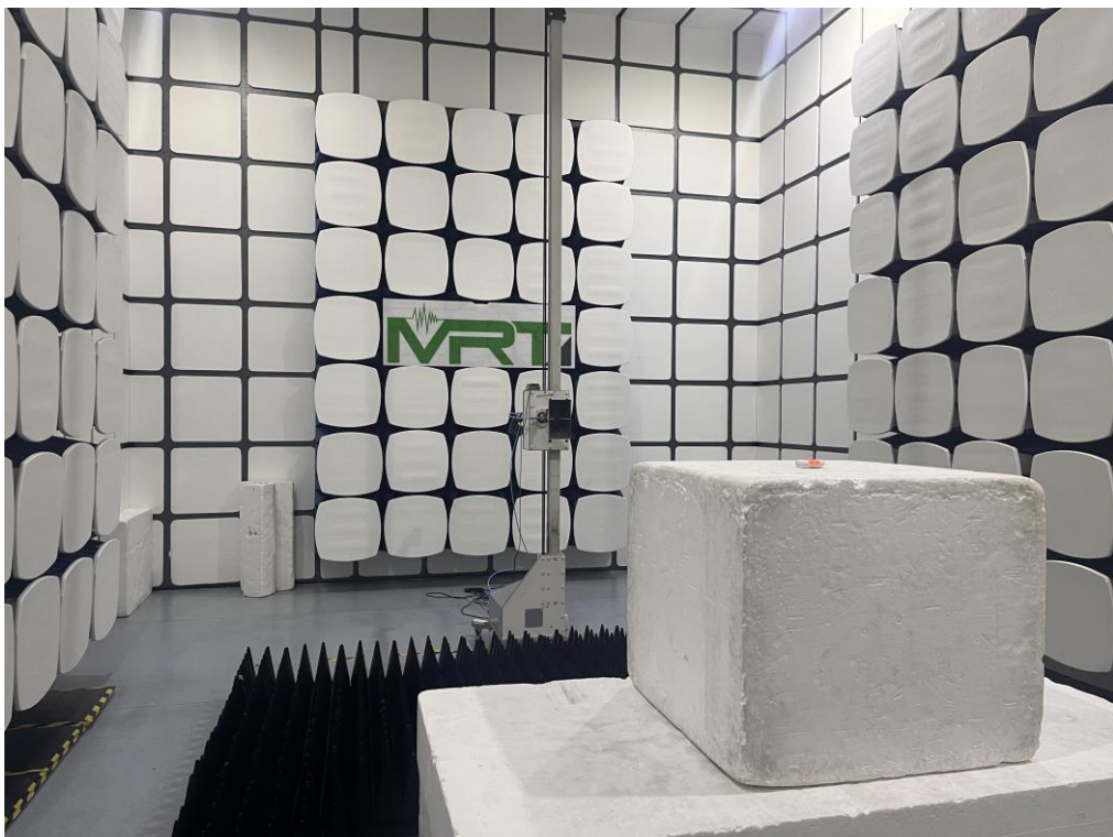
Description: Radiated Restricted Band Edge Test Setup for BLE
