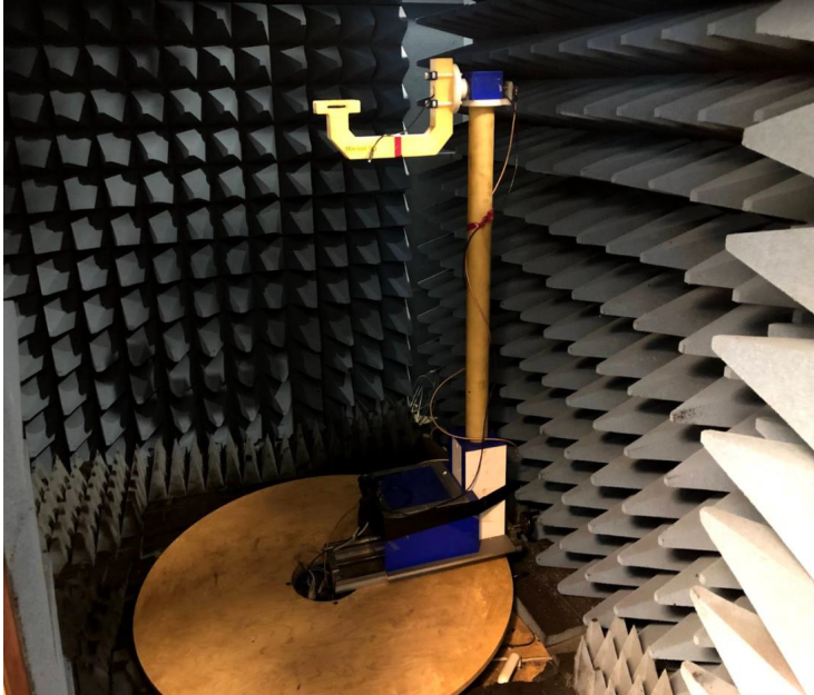
Figure 4. Receiving antenna in the anechoic chamber.
