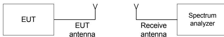
Figure 7.7.1 Band edge emission test setup
