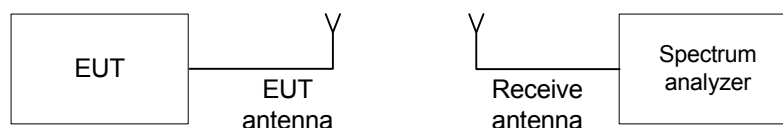
Figure 7.1.1 The 6 dB bandwidth test setup
