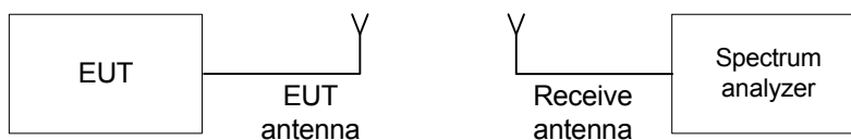
Figure 7.2.1 Carrier frequency separation test setup
