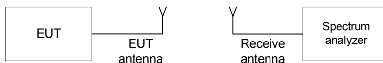
Figure 7.1.1 The 20 dB bandwidth test setup
