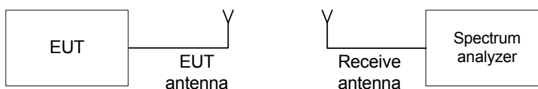
Figure 7.3.1 Hopping frequencies test setup
