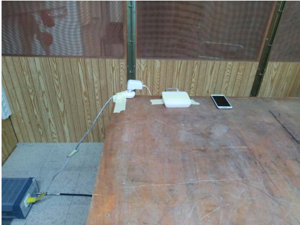
Photograph No.8 Setup for conducted emission measurements on AC power lines
