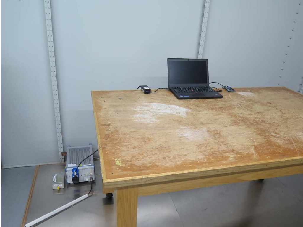
Line conducted emission (front view) (Data transfer)
