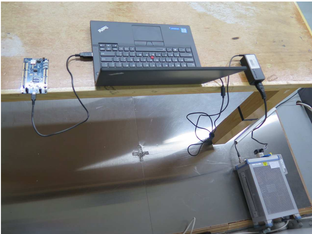
Line conducted emission (back view) (Data transfer)
