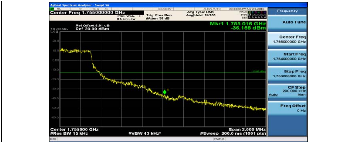
(Channel Bandwidth: 1.4 MHz)_HCH_16QAM_3RB#2
