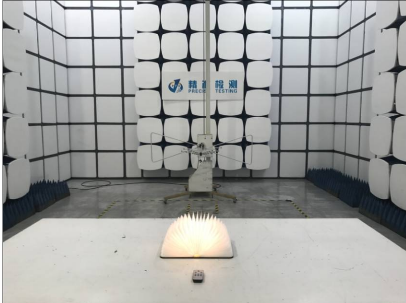
Radiated Spurious Emissions Test Frequency From 30MHz-1000MHz
