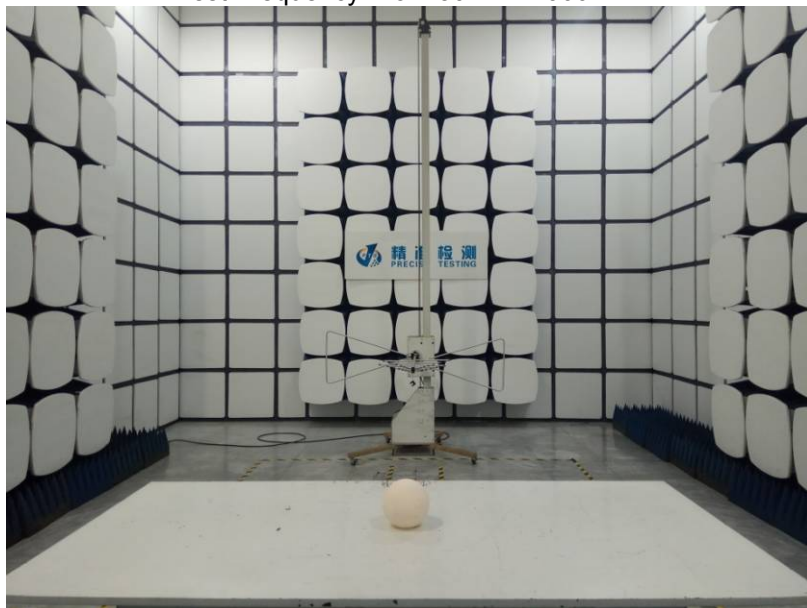
Radiated Spurious Emissions Test Frequency From 30MHz-1000MHz
