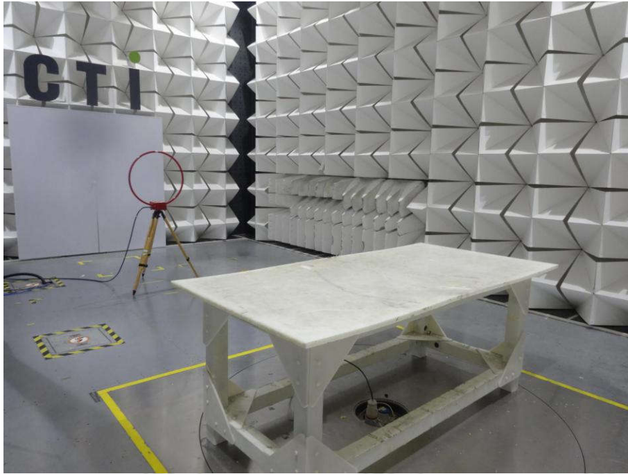
Radiated spurious emission Test Setup-1(Below 30MHz)
