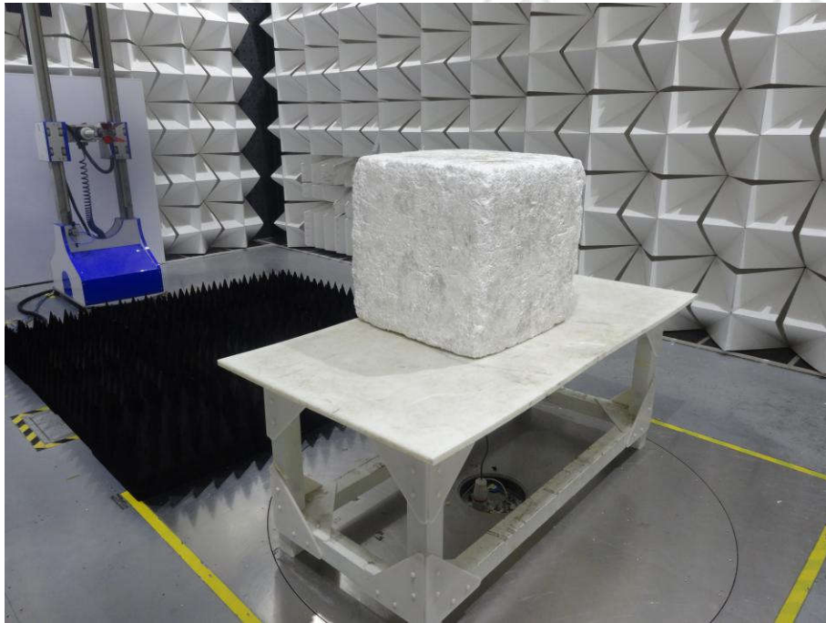
Radiated spurious emission Test Setup-3(Above 1GHz)
