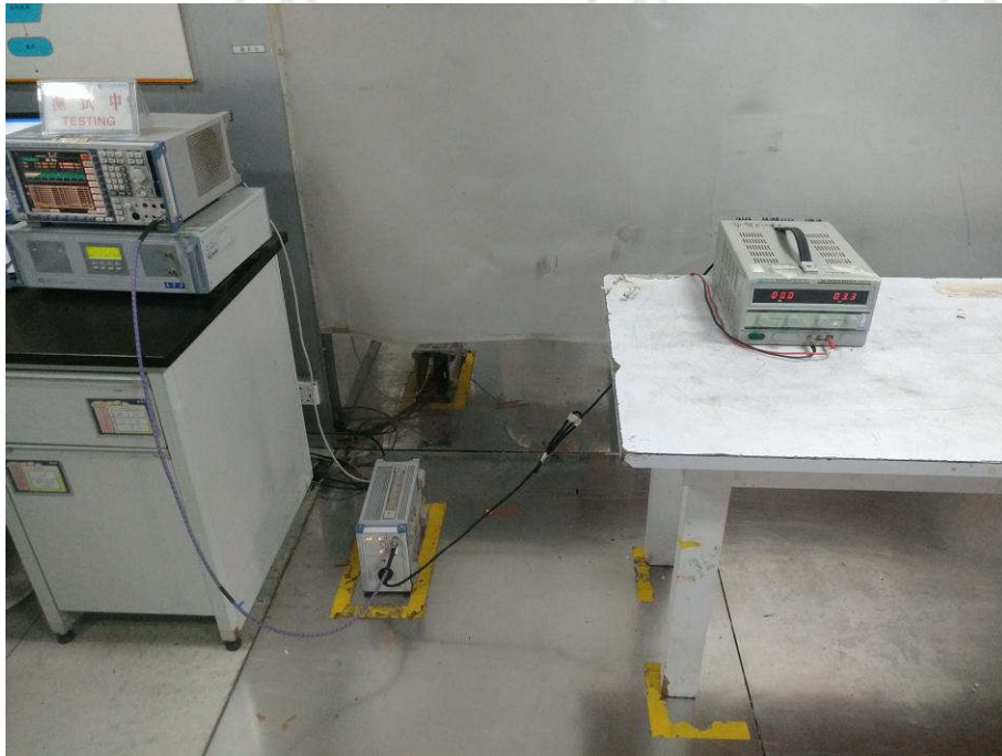
Conducted emissions Test Setup
