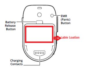
Label is located in the battery compartment, The paste is firm and the product battery is detachable.
