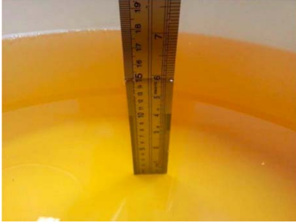
Photo 7: Tissue Simulant Liquid for Head 2450
