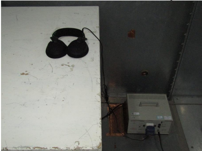
Measurement of Conducted Emission Test Set Up
