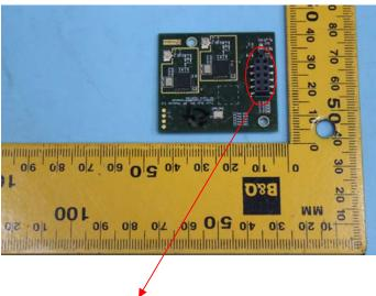
The 10 hole jack on the module is connected to the ten pins on the host device and communicates with each other (The installed host needs a ten pins connector)
