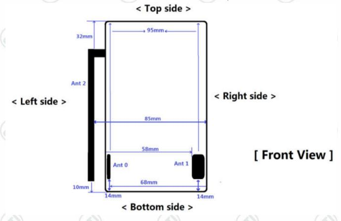
The SAR measurement positions of each side are as below:
